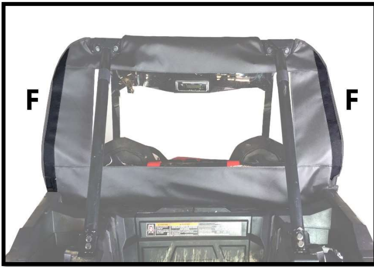
Figure 8: You will attach tabs F to Velcro strips sewn on to the back panel.
