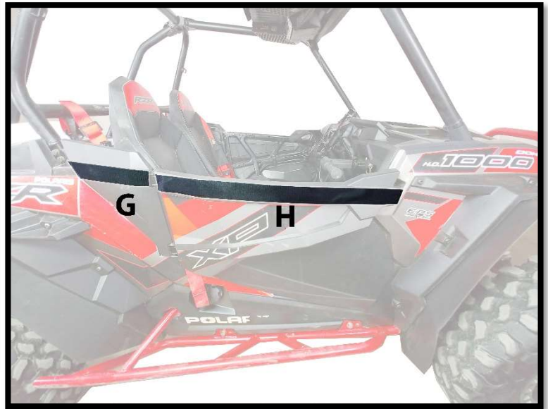
Figure 9: SHOWS PLACEMENT OF 11" AND 32" VECLRO STRIPS (G AND H). PLACE ON EITHER SIDE
