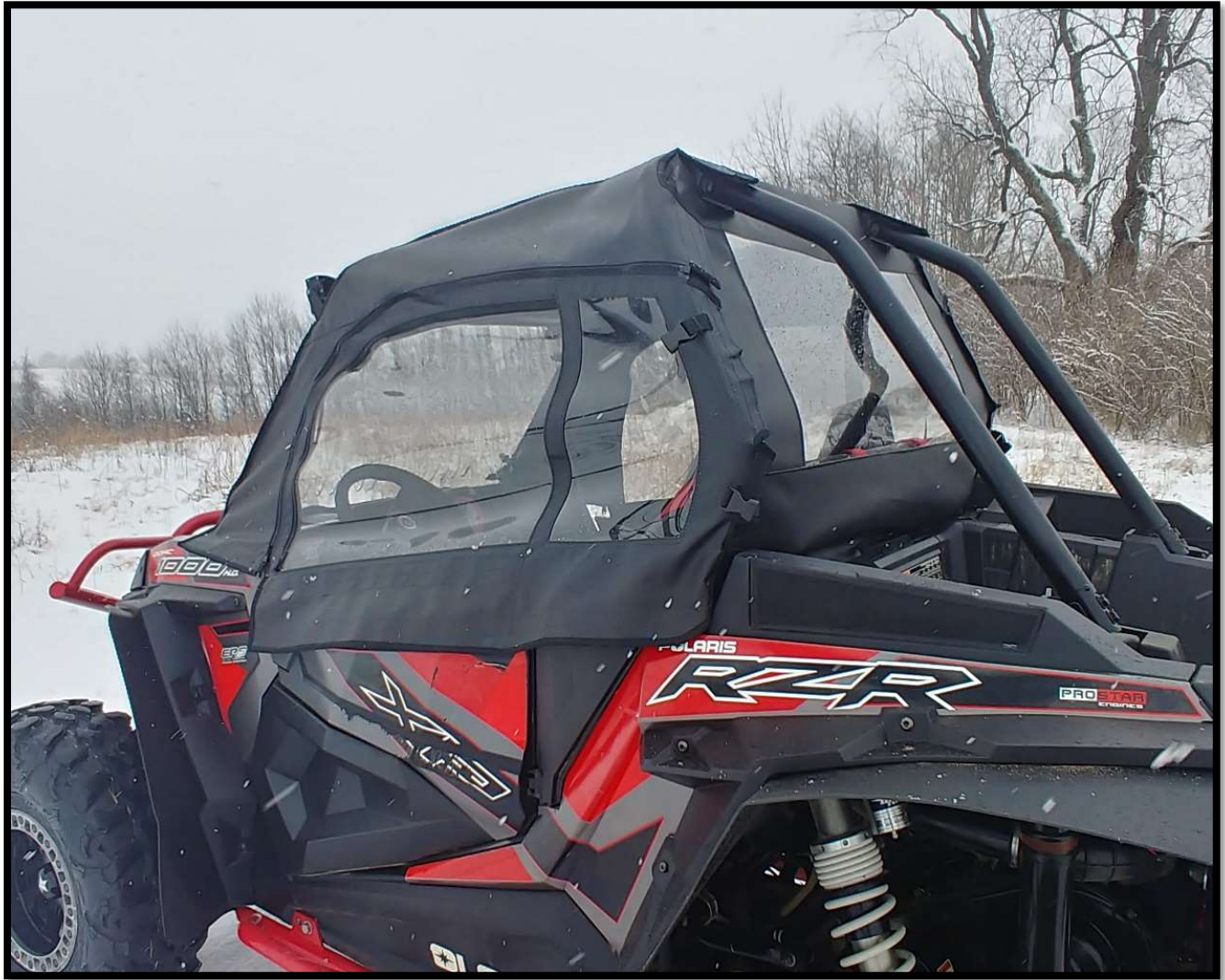
Figure 12: Upon completion of installation, your door kit will resemble the above photo. Door kit should be smooth and fit tight.
