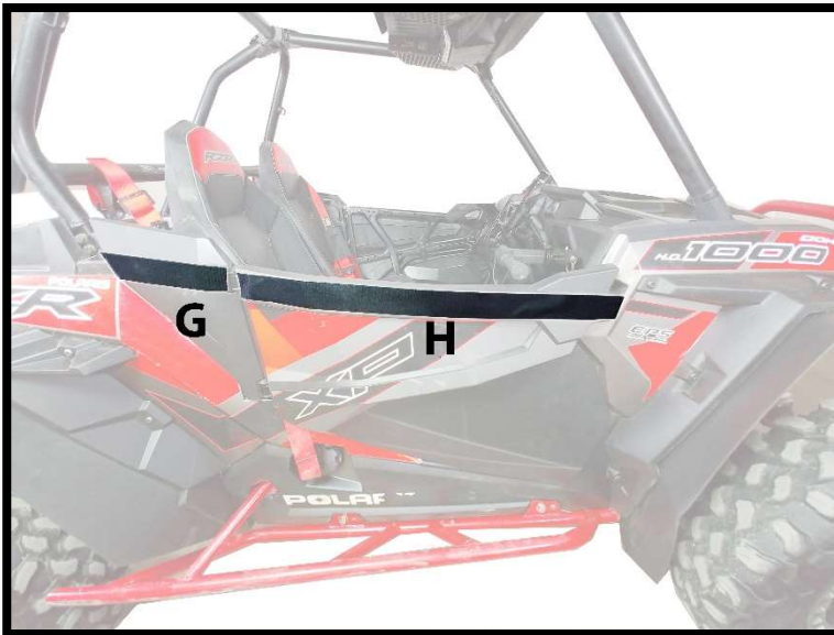
Figure 9: SHOWS PLACEMENT OF 11" AND 32" VECLRO STRIPS (G AND H). PLACE ON EITHER SIDE
