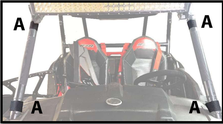
Figure 1: SHOWS POSITON OF 6" VELCRO STRIPS (A)
