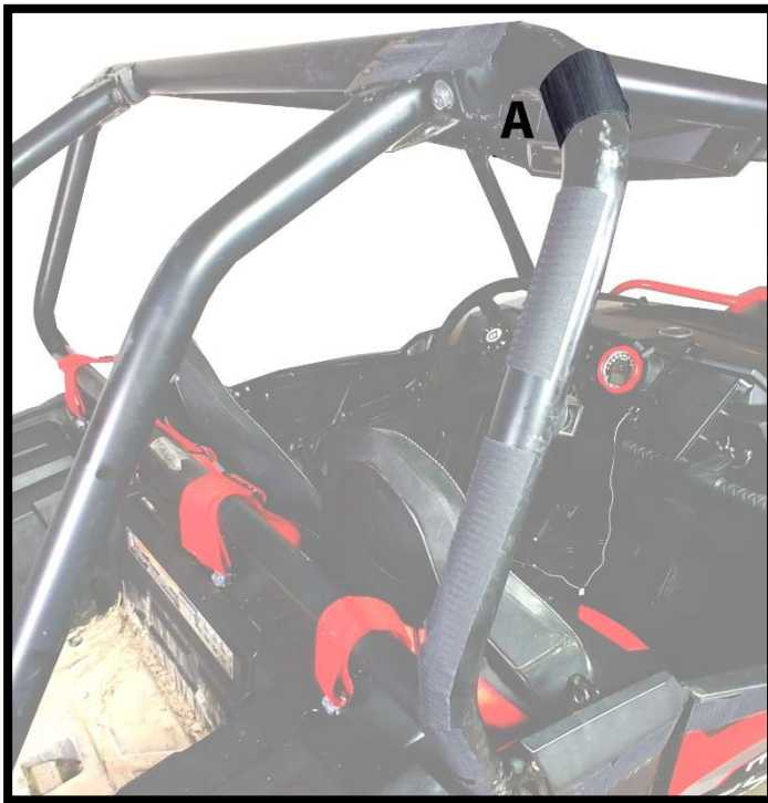
Figure 3: SHOWS PLACEMENT OF 6" VELCRO STRIPS (A). PLACE ON EITHER SIDE.
