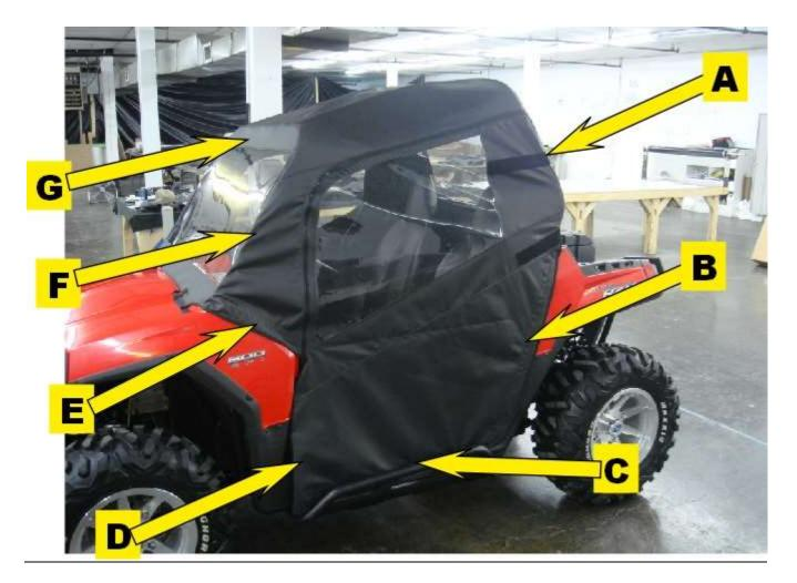
Step 4: With the exception of the 2-30" Velcro strips for the front roll bars (reference F), remove the backing and apply the adhesive Velcro strips as indicated in the ADHESIVE VELCRO KIT CONTENTS AND PLACEMENT table on page 1.
