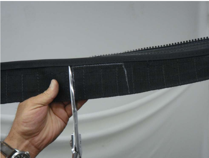
Figure 7.2 – Cut a 2” section out around where your clamps will be positioned on the Velcro Tab – be careful not to cut the binding
