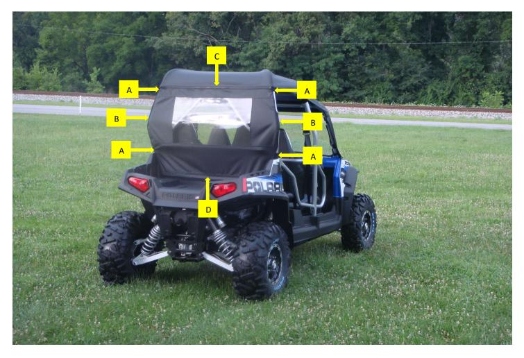
**Step 4:** Re-position the back on the enclosure as needed to square the enclosure to the rollcage. Attach the enclosure to the adhesive Velcro hook in the following order:
