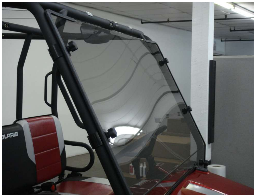
Figure 3.2 - place clamps at appropriate locations on the front Roll Bar uprights to match the windshield hole locations.
