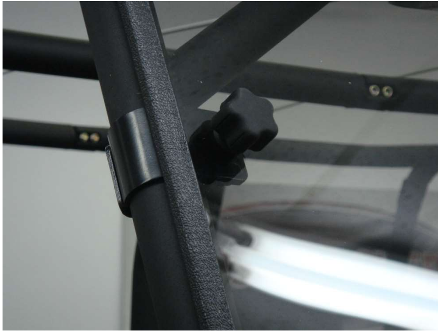
Figure 5.2 - When Knobs are tightened they should hold the flat side of the Clamp flat against the inside of the Windshield
