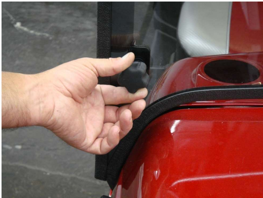
Figure 5.1 – tighten all Quick Connect Knobs
