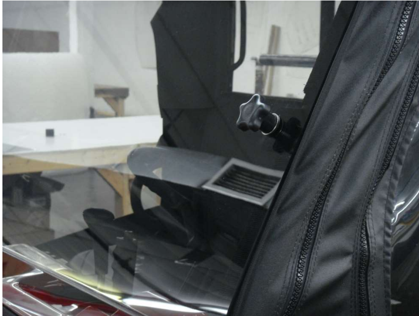
7.1 – Adjust binding edges against the edge of the Lexan Windshield
