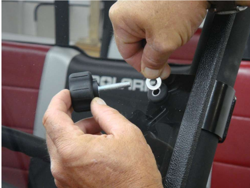
Figure 4.1 - align windshield and clamps then replace knobs and washers through the windshield.
