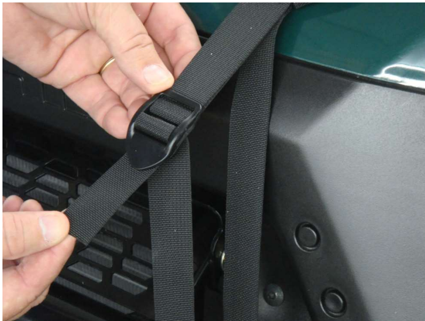
- thread front hood straps through the buckles
