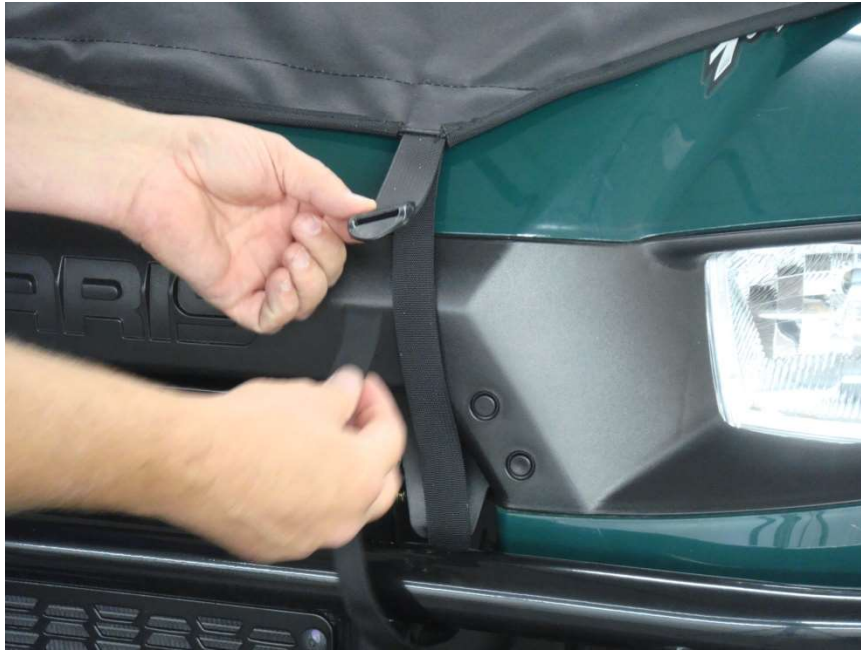
Run front hood straps around front bumper
