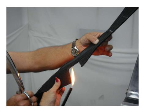
Figure 8.4 – Seal Frayed Tab thread at the cut area using a lighter
