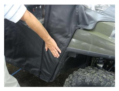
Figure 9.3 – attach Door Front Cowl Panel Enclosure 24 ½" Velcro Tabs
