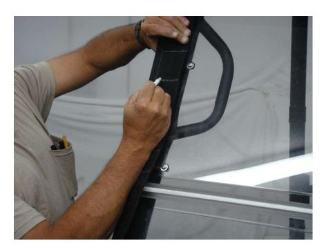
Figure 8.2 - Mark windshield tabs where hard windshield clamps are located along the windshield Roll Bar
