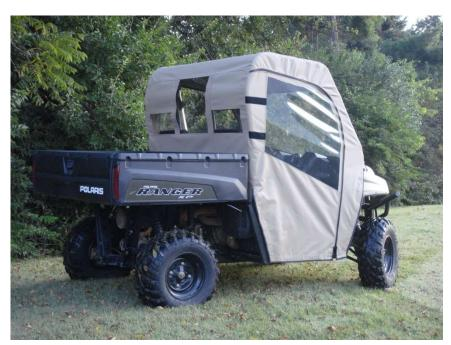
Figure 10.1 – Repeat Steps 8 and 9 until the enclosure fits snuggly to the vehicle roll bar cab
