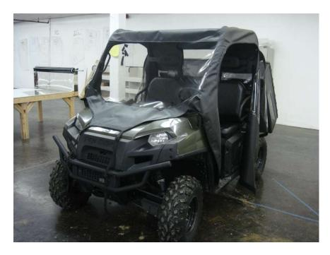
Figure 6.1 - place enclosure on vehicle cab roll bar structure - align enclosure seams with center of roll bars
