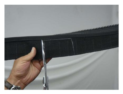
Figure 8.3 – Cut the Tab being very careful not to cut the binding at the edge
