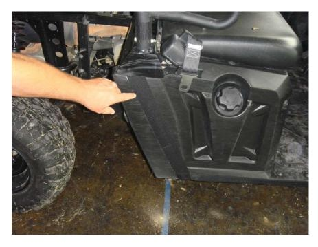
Figure 3.1 - attach 18 ½" Velcro Strips vertically along the Rear Door Panel
