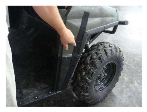
Figure 4.1 – attach 24 ½" Velcro Strips vertically along the Front Cowl Panel
