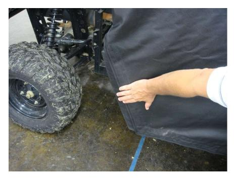
Figure 9.1 – attach Door Rear Panel Enclosure 18 %" Velcro Tabs
