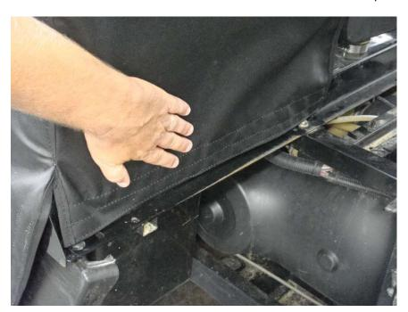
Figure 7.1 - square rear of enclosure to cab and attach rear enclosure Velcro tab to installed Velcro strips
