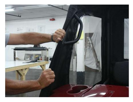
Figure 8.1 – attach Windshield Roll Bar post Velcro Tabs to installed 28" and 9" Velcro Strips
