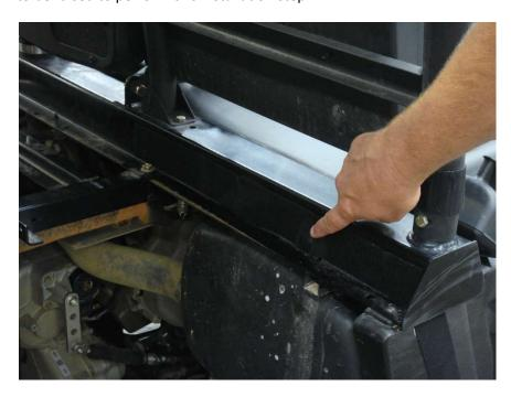
Figure 2.1 – attach 21" and 17" Velcro strips to the Rear Cab Frame
