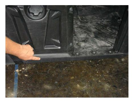
Figure 5.1 – attach 28" Velcro Strips horizontally along the door Rocker Panel – align the top side and fold the bottom 1" underneath the Rocker Panel
