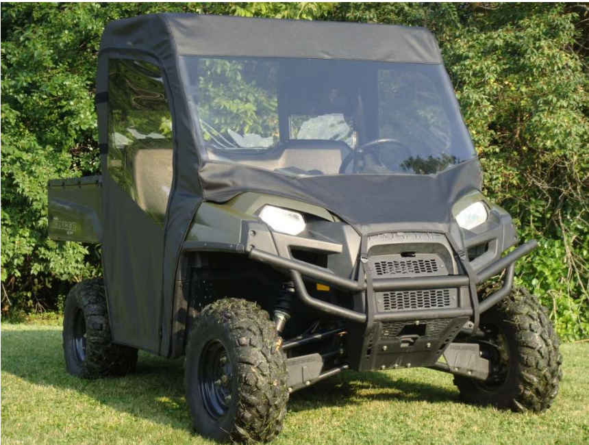
Figure 13.1 – Repeat Steps 10, 11 and 12 until the enclosure fits snugly to the vehicle roll bar cab and windows are tight
