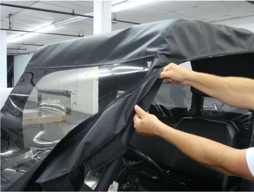
Figure 10.1 - attach top front Windshield roll bar 8" Velcro tabs
