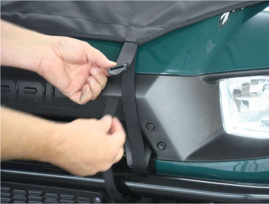
Figure 9.1 - run front hood straps around front bumper
