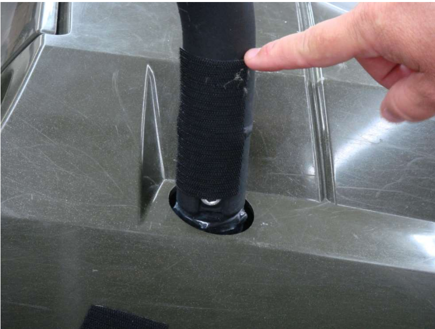
Figure 3.1 - attach 4” Velcro strips vertically at the front roll bar post cowl opening
