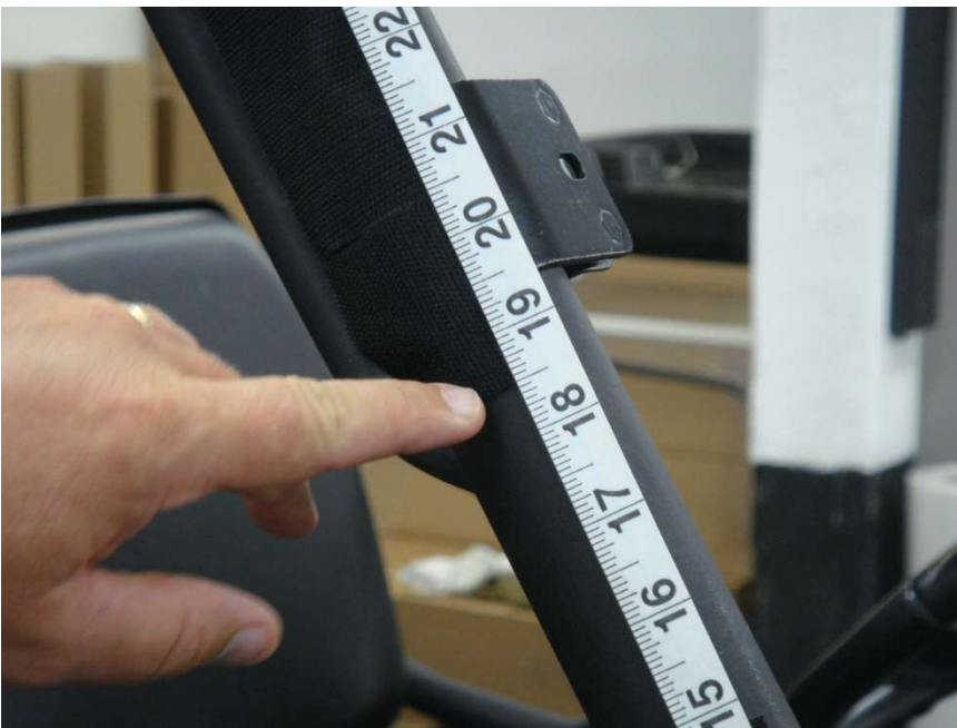
Figure 3.3 - attach 8" Velcro Strips vertically 18 1/2" above the front roll bar post cowl opening
