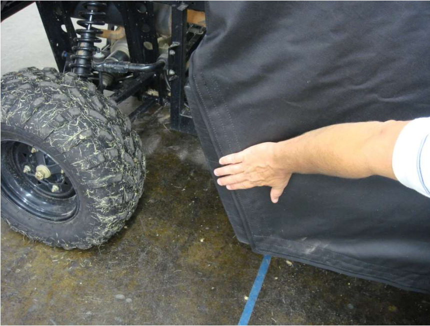
Figure 12.1 – attach Door Rear Panel Enclosure 18 ½" Velcro Tabs
