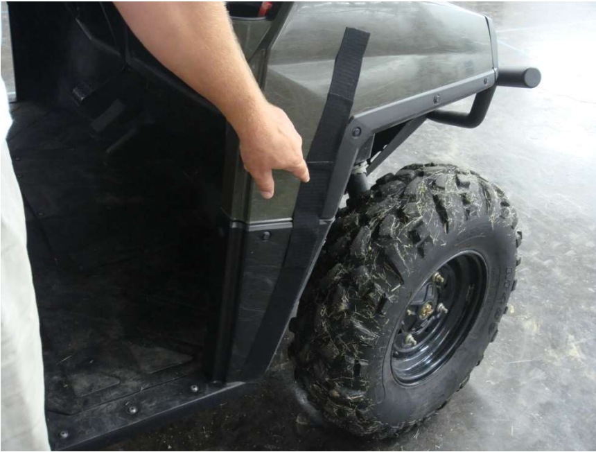
Figure 5.1 – attach 24 ½" Velcro Strips vertically along the lower Front Cowl Panel
