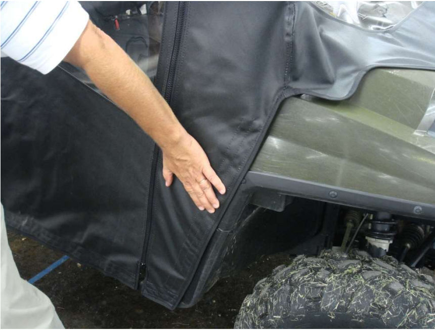
Figure 12.3 – attach Door Front Cowl Panel Enclosure 24½” & lower front 4 ½” Velcro Tabs
