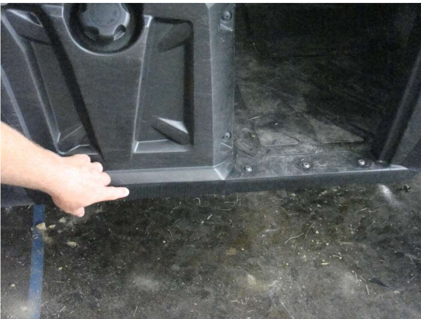
Figure 6.1 – attach 28" Velcro Strips horizontally along the door Rocker Panel
