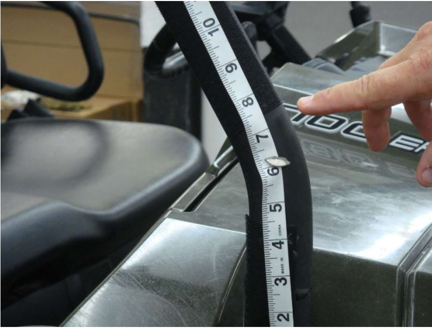
Figure 3.2 - attach 6" Velcro strips vertically 7 1/2" above the front roll bar post cowl opening
