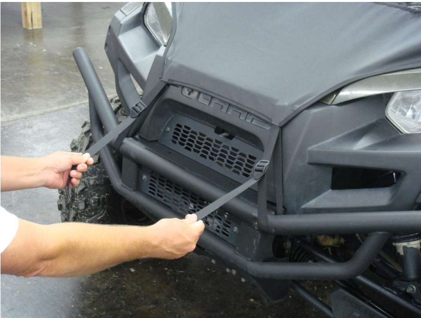
Figure 11.1 – Fully tighten both Hood Straps pulling downward on both at the same time
