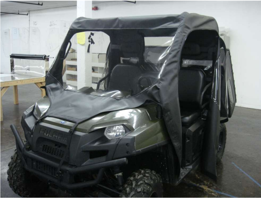
Figure 7.1 - place enclosure on vehicle cab roll bar structure – align enclosure seams with center of roll bars
