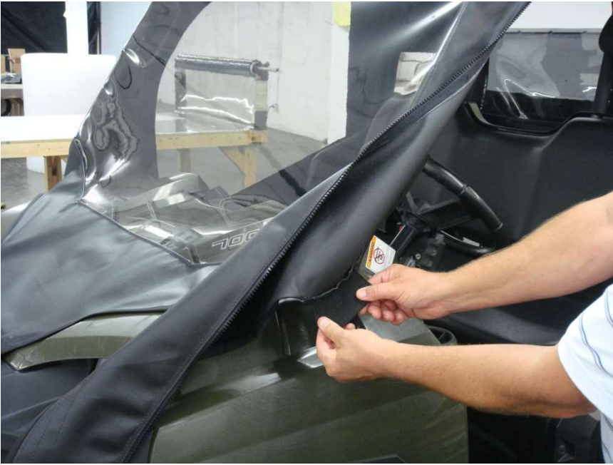
Figure 10.3 - attach bottom front Windshield roll bar 4" Velcro tabs
