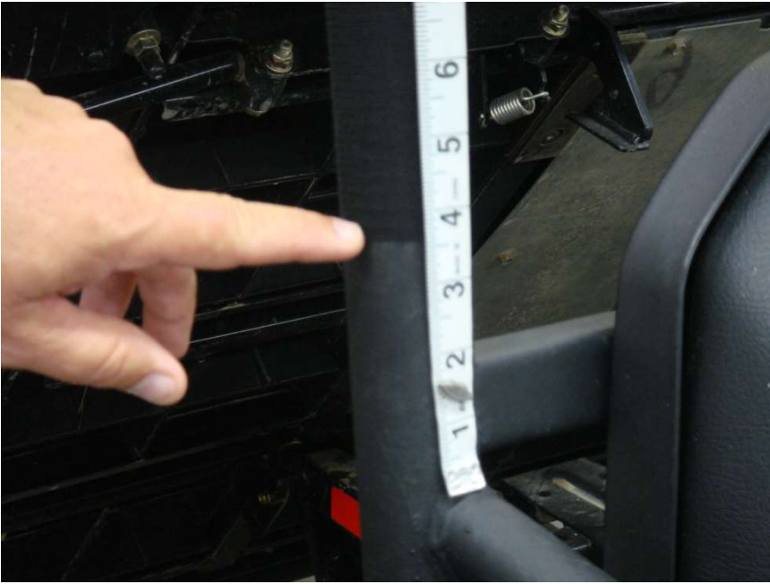
Figure 3.4 – attach Rear Roll Bar upright Velcro strips 4" above the arm rest bar
