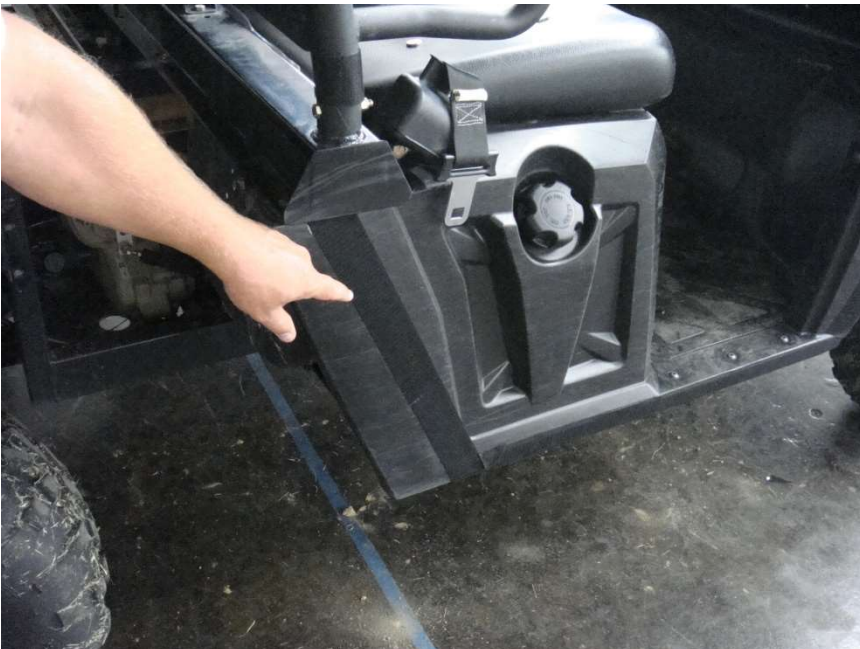
Figure 4.1 - attach 18 ½" Velcro Strips vertically along the lower Rear Door Panel
