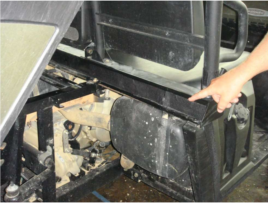
Figure 2.1 – attach 21” Velcro strip to the Rear Cab Frame on Passenger and Drive side; attach 17” Velcro Strip above breather at center
