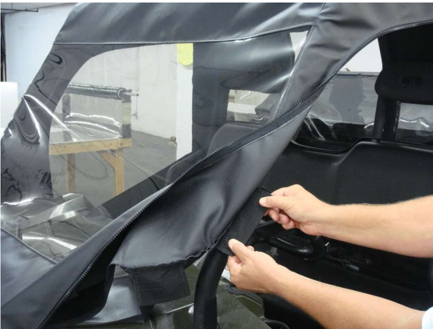
Figure 10.2 - attach middle front Windshield roll bar 6" Velcro tabs
