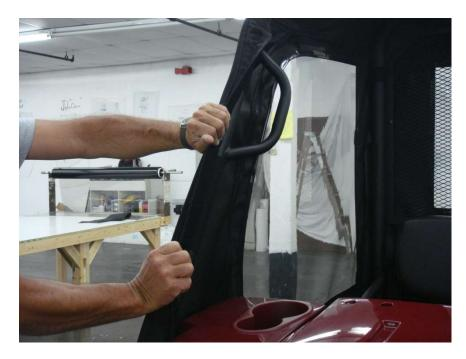
Figure 10.1 – attach Windshield Roll Bar post Velcro Tabs to installed 28" and 9" Velcro Strips
