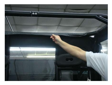
Figure 9.4 – attach 49" Rear Top Roll Bar Frame Velcro Tabs
