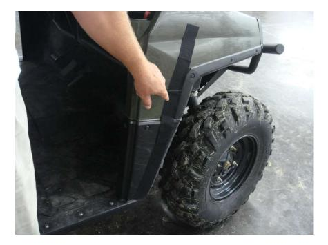
Figure 4.1 – attach 24 1/2" Velcro Strips vertically along the Front Cowl Panel
