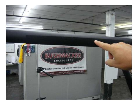
Figure 6.1 - adhere the 49" Rear and 15" Side Roll Bar Cross-member Velcro Strips
