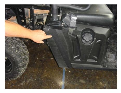
Figure 3.1 - attach 18 1/2" Velcro Strips vertically along the Rear Door Panel
