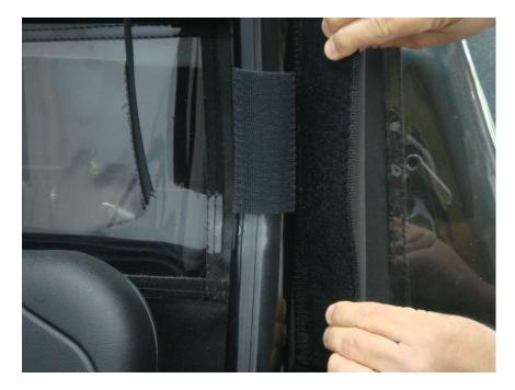
Figure 9.2 – attach 8" rear Roll Bar upright tabs
