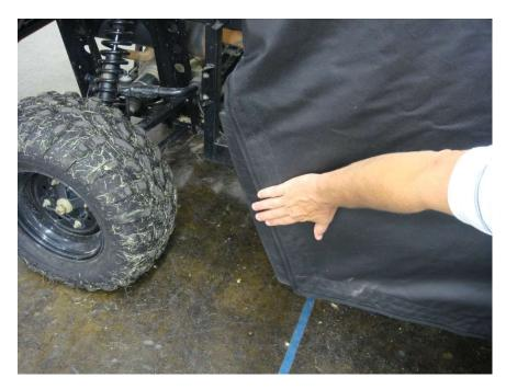
Figure 11.1 – attach Door Rear Panel Enclosure 18 ½" and 4 ½" Velcro Tabs
