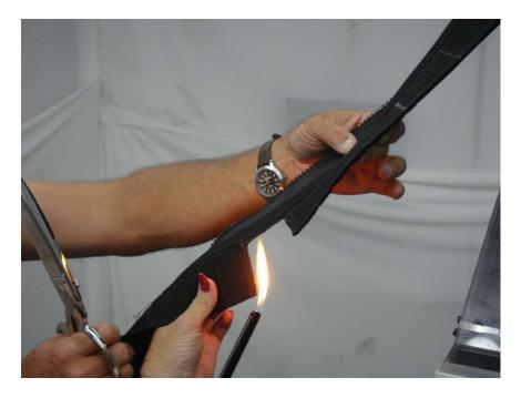
Figure 10.4 – Seal Frayed Tab thread at the cut area using a lighter
