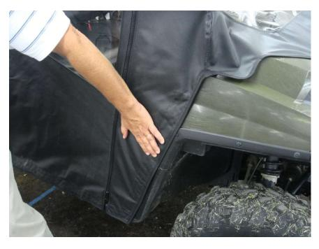
Figure 11.3 – attach Door Front Cowl Panel Enclosure 24 1/2" Velcro Tabs
