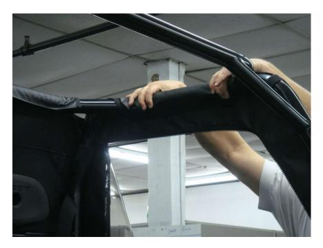
Figure 9.3 – attach 15" Door Top Roll Bar Frame Velcro Tabs
