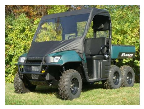
Figure 9.1 – Repeat Steps 5, 6, 7 & 8 until the enclosure fits snuggly to the vehicle roll bar cab and windshield is tight
