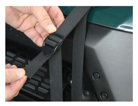
Figure 6.2 - thread front hood straps through the buckles
