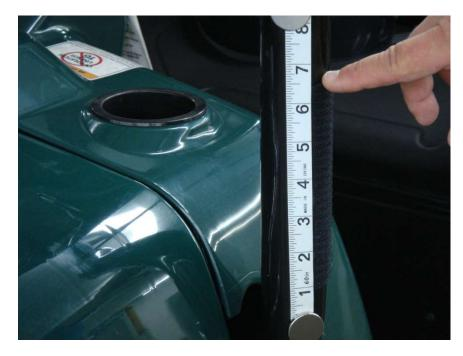
Figure 3.1 - attach 5" Velcro strips vertically approx 6 1/2" above the front roll bar post cowl opening
