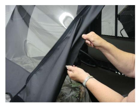
Figure 7.2 - attach middle front Windshield roll bar 10" Velcro tabs
