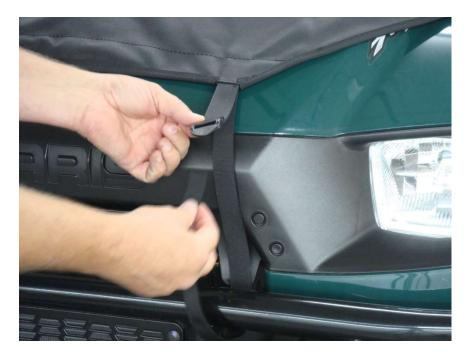
Figure 6.1 - run front hood straps around front bumper
