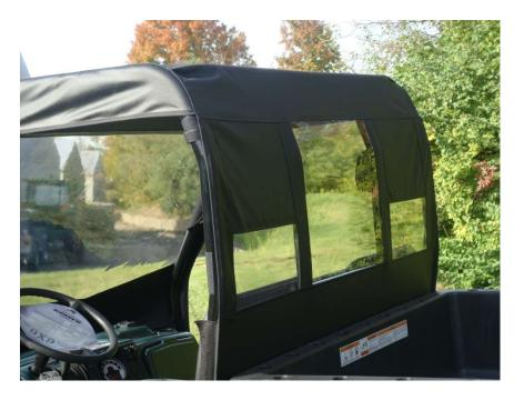
Figure 9.2 – Rear windows should be tight across the back of the Cab
