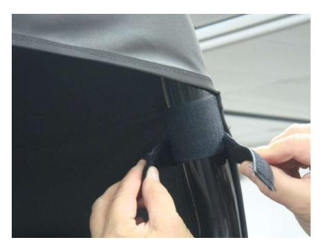
Figure 5.3 – attach rear Roll Bar upright top horizontal 6" Velcro Tabs
