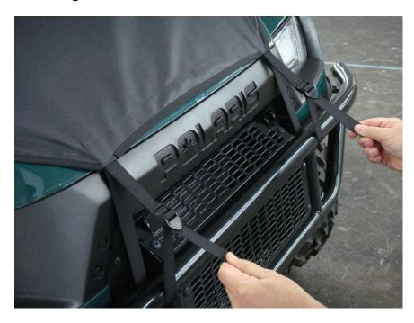
Figure 8.1 – Fully tighten both Hood Straps pulling downward on both at the same time
