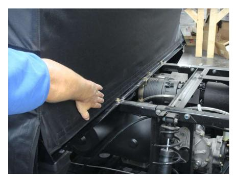
Figure 5.1 - square rear of enclosure to cab and attach rear enclosure Velcro tab to installed Velcro strip
