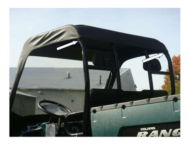
Figure 3.1 - attach 6" Velcro strips horizontally approx 1" below the Velcro straps sewn into the top corners.
