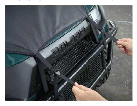
Fully tighten both Hood Straps pulling downward on both at the same time
