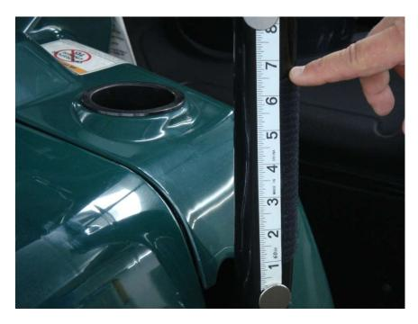
Figure 3.1 - attach 5" Velcro strips vertically approx 6 ½" above the front roll bar post cowl opening
