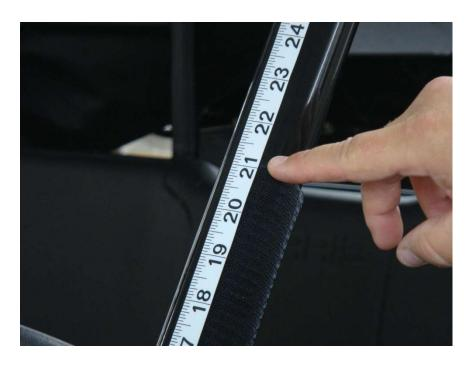
Figure 3.2 - attach 10" Velcro strips vertically approx 21" above the front roll bar post cowl opening
