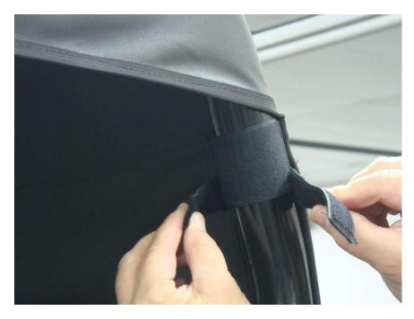
Figure 4.1 – attach rear Roll Bar upright top horizontal 6" Velcro Tabs
