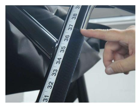
Figure 3.3 - attach 10" Velcro Strips vertically approx 37" above the front roll bar post cowl opening
