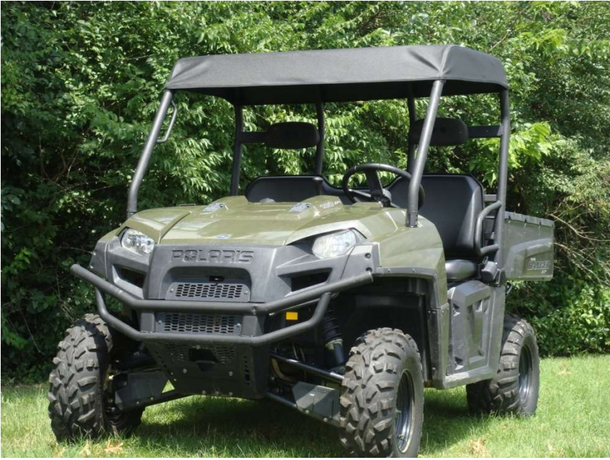
Figure 6.1 - re-tighten each Velcro Tab until the Top Cap is tight on all sides and no major wrinkles are showing.
