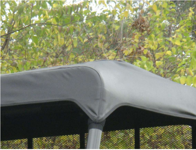
Figure 4.1 - Wrap 6" adhesive hook strips around roll bar. Wrap the double-sided straps at each corner around the adhesive strips.
