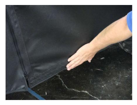
Figure 11.2 – attach Door Rocker Panel Enclosure 27" Velcro Tabs
