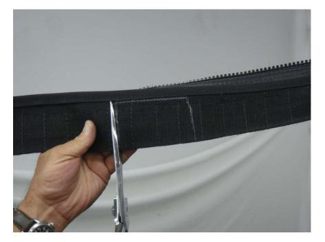
Figure 10.3 – Cut out the Tab at the Clamp location being very careful not to cut the binding at the edge
