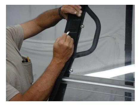
Figure 10.2 – Mark enclosure windshield tabs where Roll Bar Clamps are located
