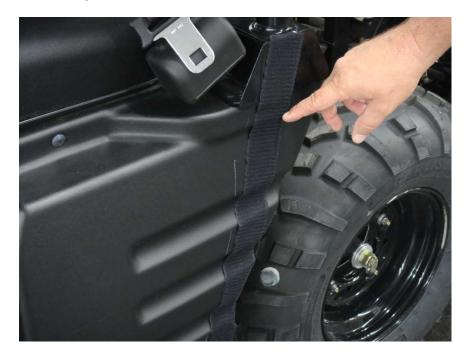
Figure 3.1 - attach 20" Velcro Strips vertically along the lower Rear Door Panel
