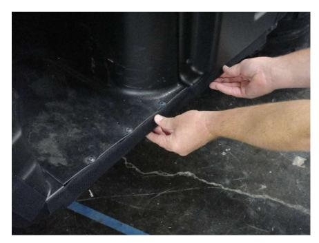
Figure 5.1 – attach 27" Velcro Strips horizontally along the door Rocker Panel – align the top side and fold the bottom 1" underneath the Rocker Panel
