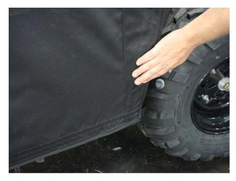
Figure 11.1 – attach Door Rear Panel Enclosure 20" Velcro Tabs
