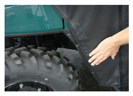
Figure 11.3 – attach Door Front Cowl Panel Enclosure 18 ½" Velcro Tabs
