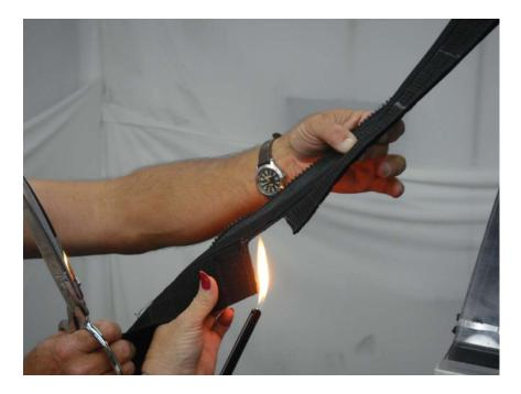
Figure 10.4 – Seal frayed Tab thread ends at the cut area using a lighter
