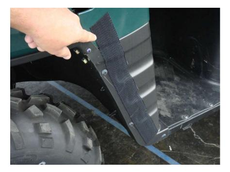
Figure 4.1 – attach 18 1/2" Velcro Strips vertically along the lower Front Cowl Panel
