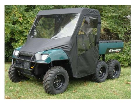
Figure 12.1 – Repeat Steps 9, 10 and 11 until the enclosure fits snuggly to the vehicle roll bar cab
