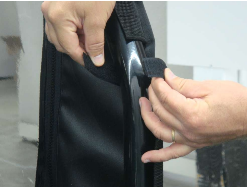
Figure 11.4 attach 6" Front Windshield Top, Middle and lower tabs around install Velcro strips
