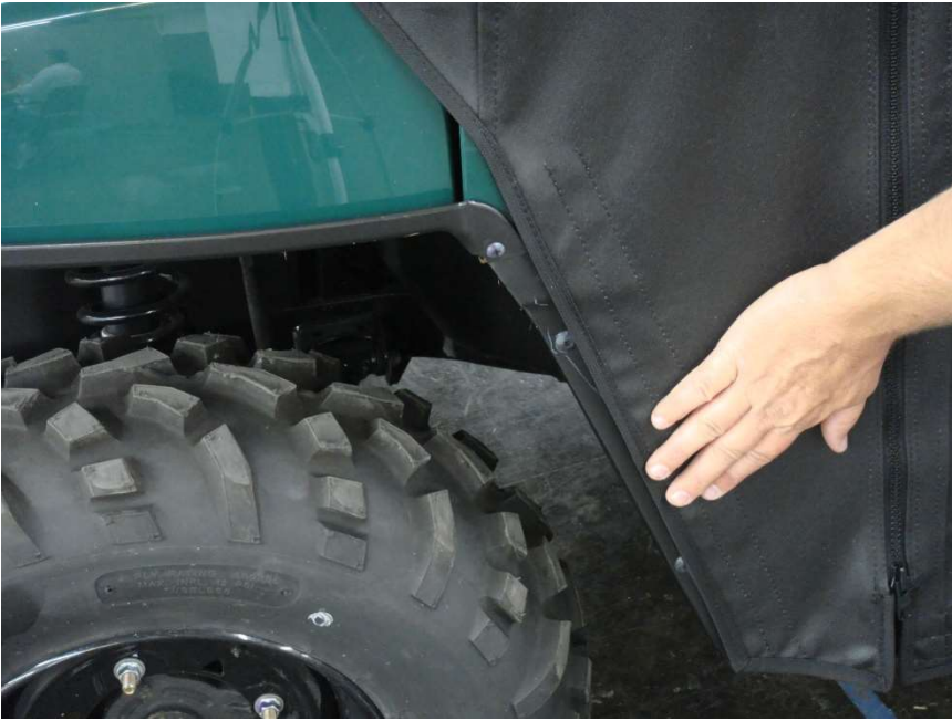
Figure 11.1 – attach Door Front Panel Enclosure 18 ½” and 10” Velcro Tabs
