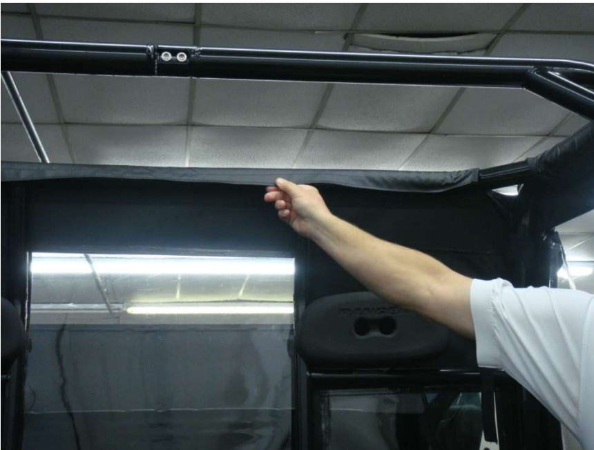
Figure 9.4 – attach 49” Rear Top Roll Bar Frame cross-member Velcro Tab
