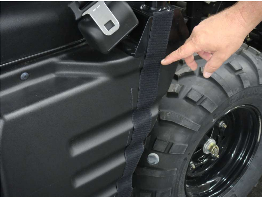
Figure 3.1 - attach 20" Velcro Strips vertically along the Rear Door Panel
