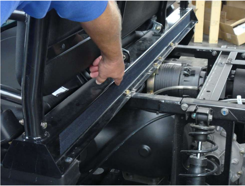
Figure 2.1 – attach 55" Velcro strip to the Rear Cab Frame
