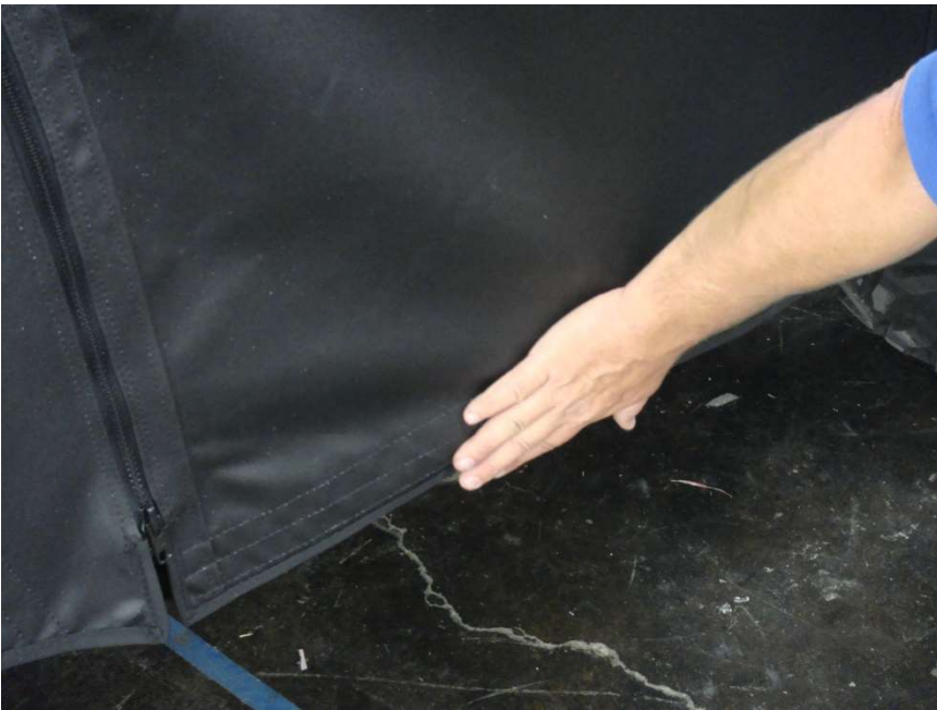
Figure 11.2 – attach Door Rocker Panel Enclosure 25” Velcro Tabs
