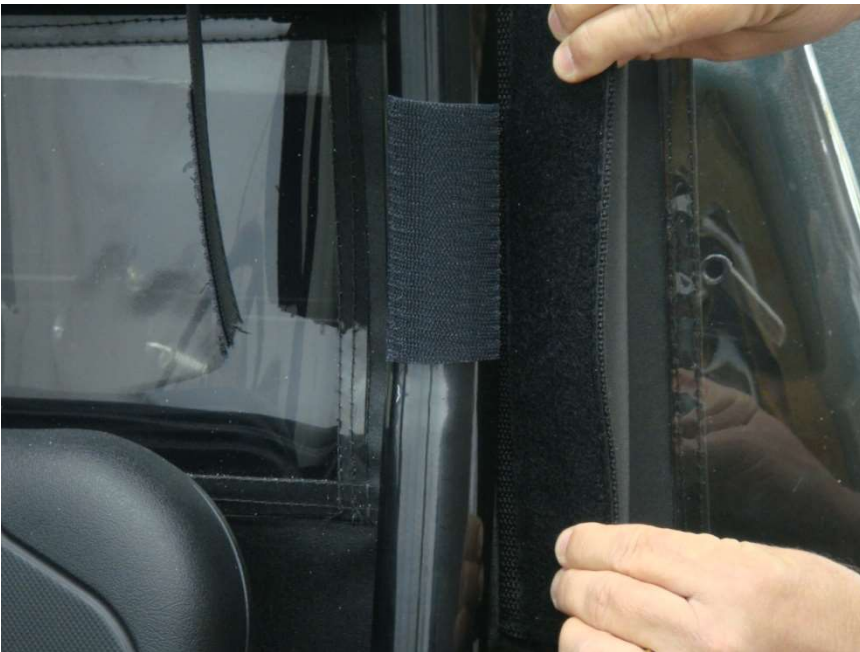
Figure 9.2 – attach 10" rear Roll Bar upright tabs
