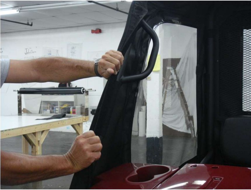
Figure 10.1 – attach Windshield Roll Bar post Velcro Tabs to installed 23” Velcro Strips
