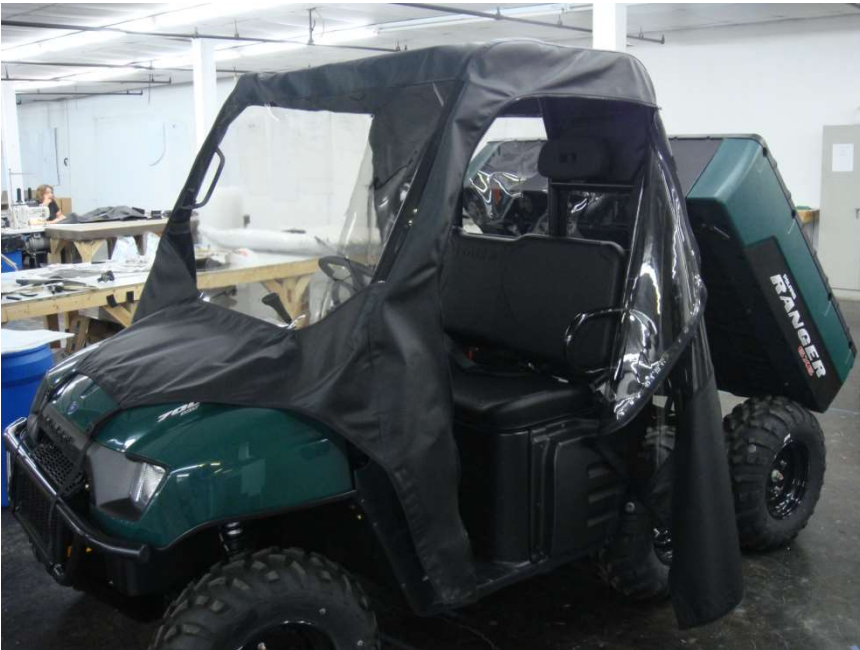
Figure 8.1 - place enclosure on vehicle cab roll bar structure – align enclosure seams with center of roll bars
