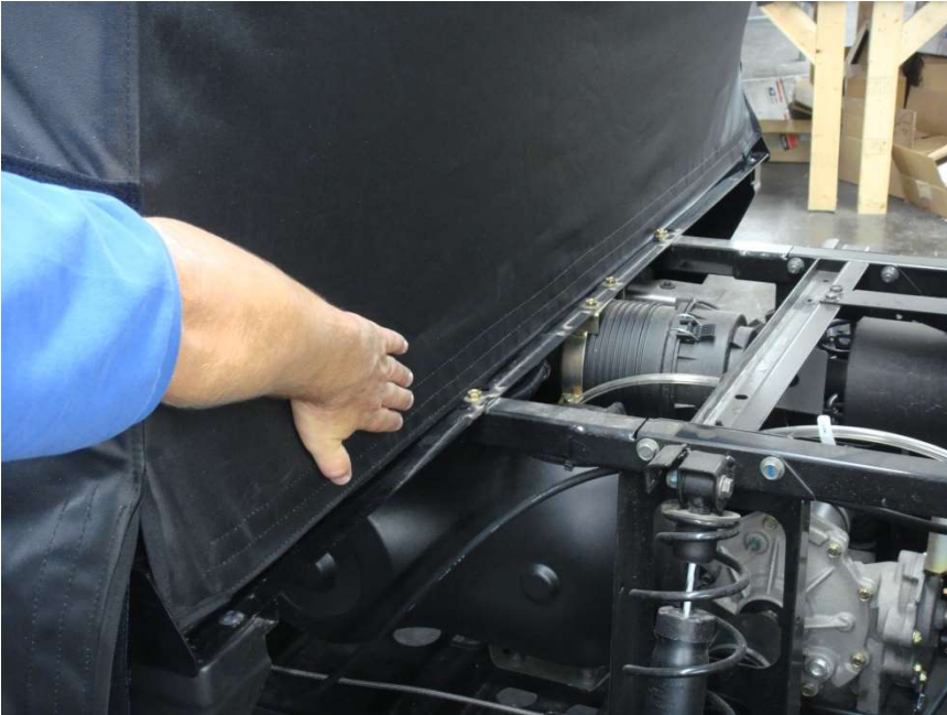
Figure 9.1 - square rear of enclosure to cab and attach rear enclosure Velcro tab to installed Velcro strip
