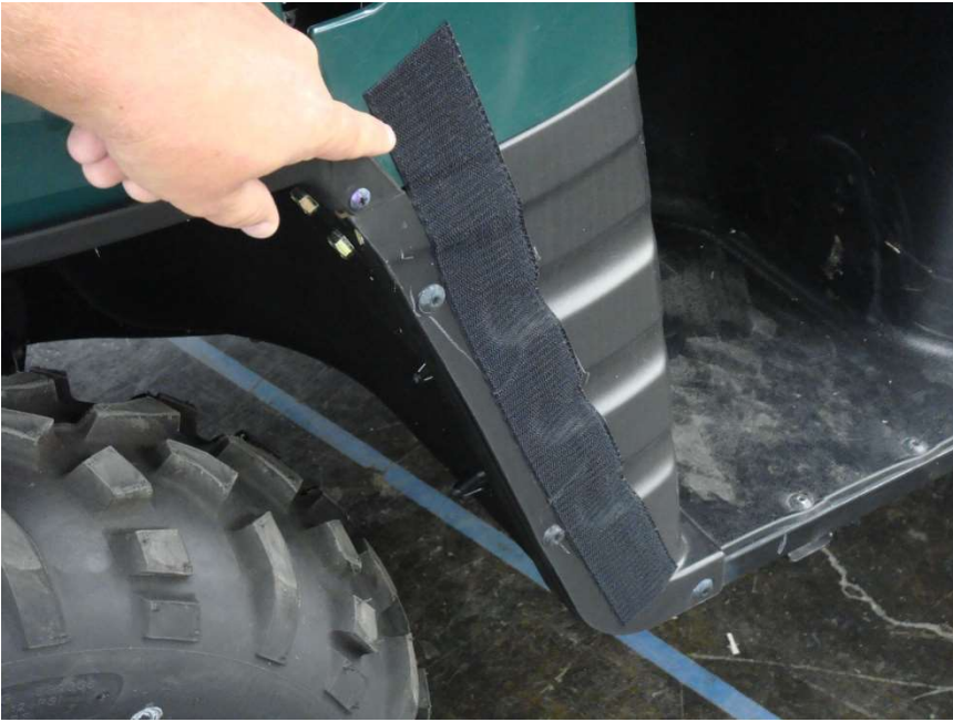
Figure 4.1 – attach 18 ½” Velcro Strips vertically along the Front Cowl Panel
