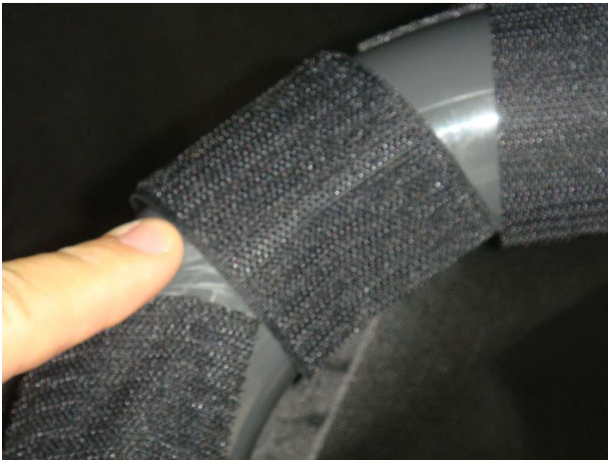
Figure 6.2 – adhere 6" Front Windshield Roll Bar post Velcro strips around the Roll Bar
