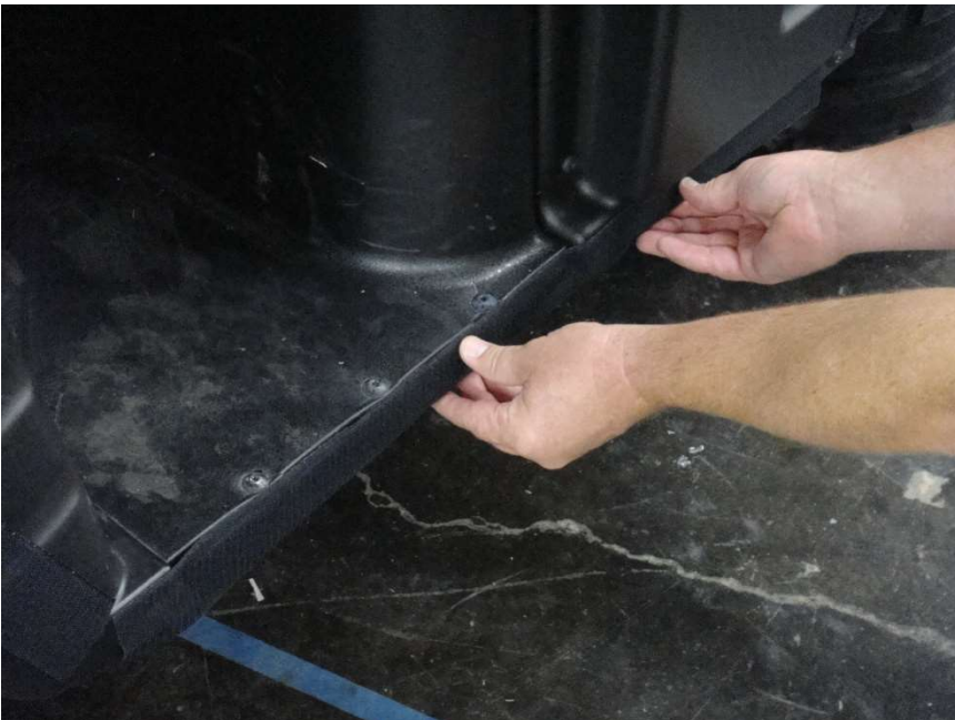
Figure 5.1 – attach 25” Velcro Strips horizontally along the door Rocker Panel
