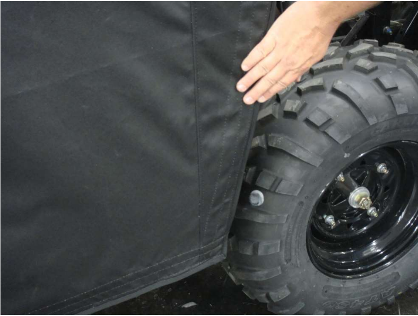
Figure 11.3 – attach Door Rear Panel Enclosure 20" Velcro Tabs
