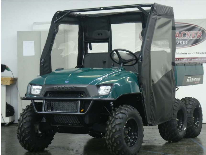
Figure 12.1 – Repeat Steps 9, 10 & 11 until the enclosure fits snugly to the vehicle roll bar cab
