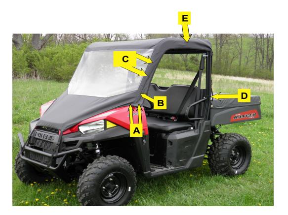
**Step 3:** After all adhesive hook strips are attached, begin attaching the enclosure to the cab frame. As you attach the hook and loop, square each panel to the frame. <u>PLEASE NOTE, FOR MAXIMUM ADHESION, ALLOW THE ADHESIVE HOOK</u> <u>TO ADHERE TO THE FRAME FOR 24 HOURS BEFORE PULLING AGAINST THE HOOK WITH THE LOOP STRIPS.</u>
