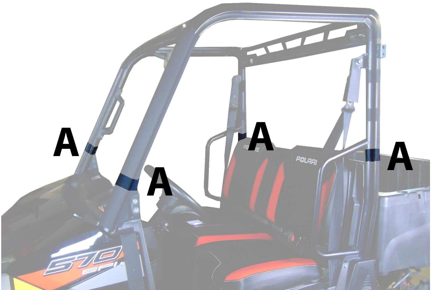
Figure 1: WRAP THESE VELCRO STRIPS AROUND THE ROLL BAR AND ATTACH DOUBLE-SIDED STRAP.
