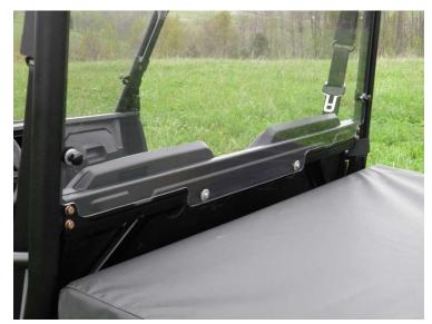
**Step 4:** As each clamp is placed into position, insert a hex head bolt thru a neoprene washer. Insert the bolt thru the back panel and thru the corresponding clamp. Insert a flat washer and lock nut onto the bolt. Only hand tighten at this time.
