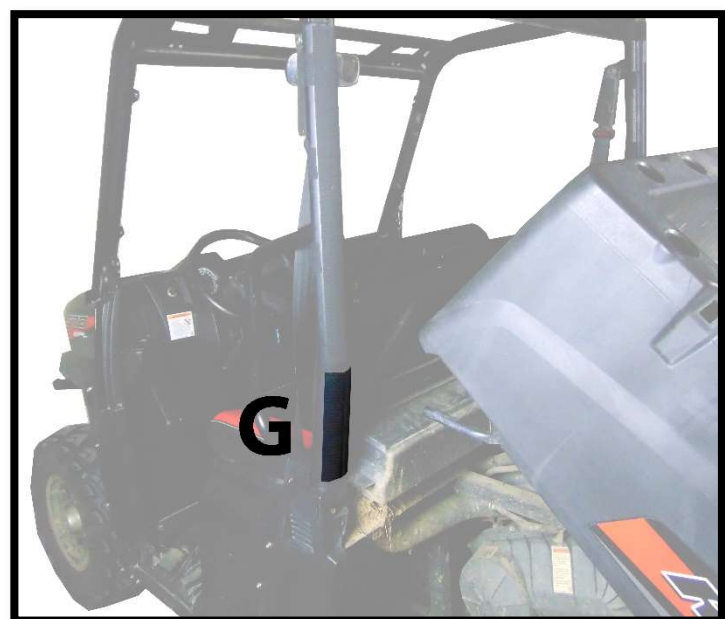
Figure 6: SHOWS PLACEMENT OF 9" VELCRO STRIPS (G)
