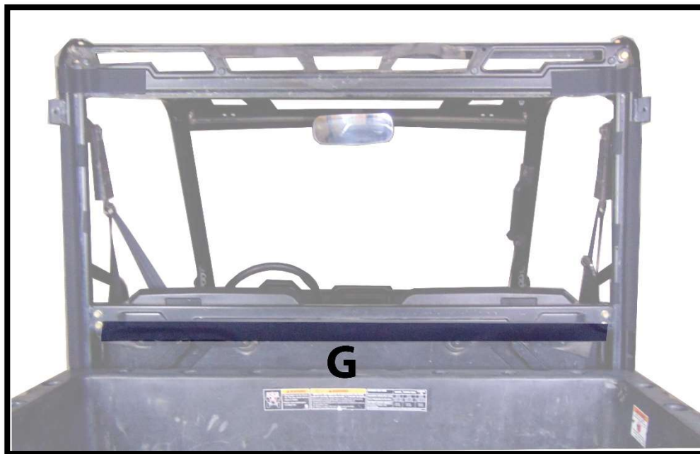
Figure 5: SHOWS PLACEMENT OF 54" VELCRO STRIP (G)
