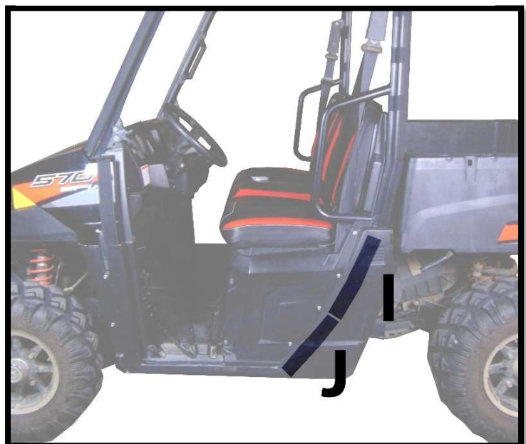
Figure 8: SHOWS PLACEMENT OF 13" VELCRO STRIPS (I AND J).
