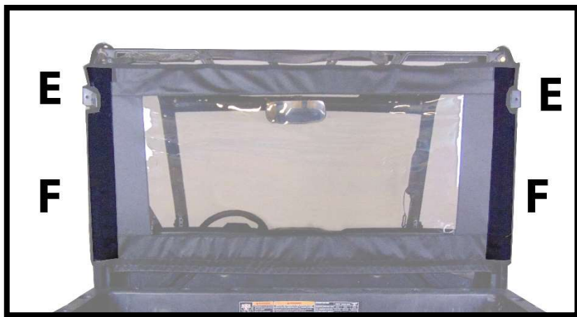
Figure 5: VELCRO FOR DOUBLE SIDED STRAPS E AND TABS F IS SEWN ON TO THE BACK PANEL
