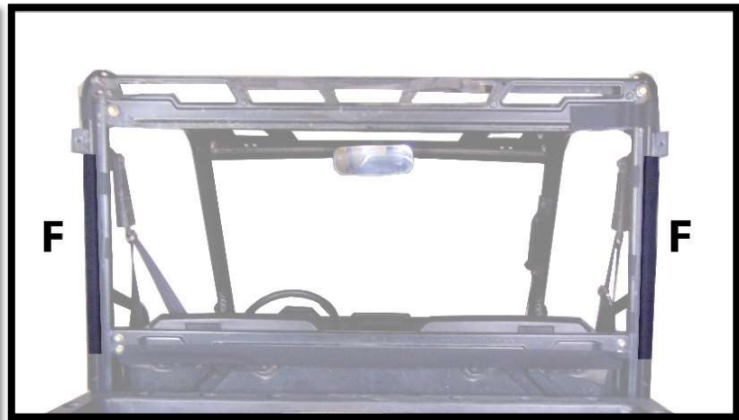
Figure 4: SHOWS PLACEMENT OF 18" VELCRO STRIPS (F).
