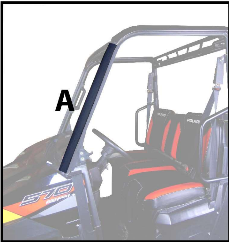
Figure 1: SHOWS PLACEMENT OF 26" VELCRO STRIPS (A) VELCRO. THE STRIP OF VELCRO SEWN ON TO THE DOOR WILL ATTACH TO THIS STRIPS.
