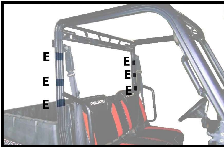
Figure 3: SHOWS PLACEMENT OF 6" VELCRO STRIPS (E)
