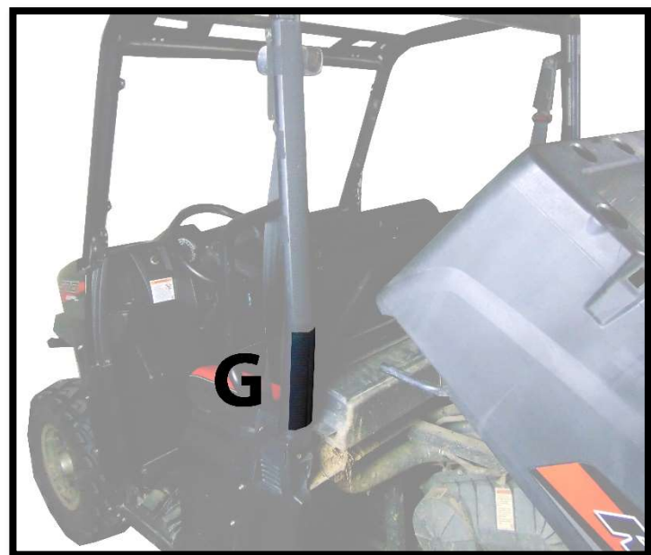
Figure 6: SHOWS PLACEMENT OF 9" VELCRO STRIPS (G)
