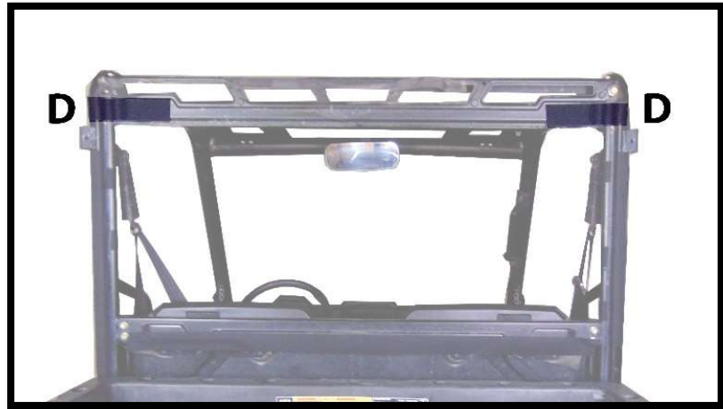
Figure 2: SHOWS PLACEMENT OF 12" VELCRO STRIPS (D).
