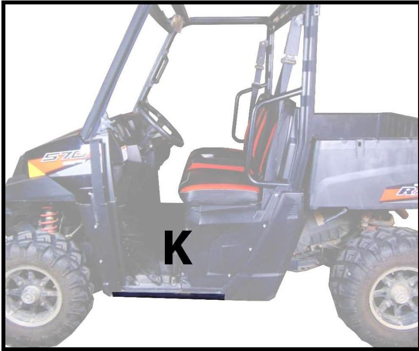
Figure 9: SHOWS PLACEMENT OF 22" VLECRO STRIPS (K)
