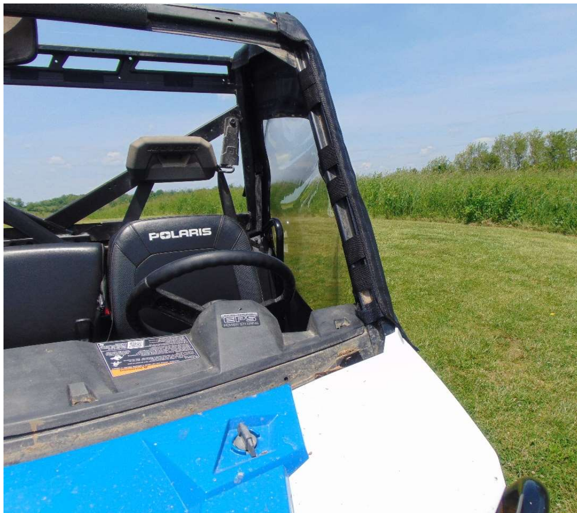
Figure 10: WHEN ATTACHING DOOR TO ADHESIVE VELCRO START WITH SIDE A. ALIGN BLACK TRIM ON THE DOOR PANEL TO THE EDGE OF THE INSET ROLL BAR. WRAP TABS AROUND THE INSIDE OF THE BAR AND ATTACH TO ADHESIVE VELCRO. CONTINUE TO ATTACH DOOR TABS AND STRAPS IN THE ORDER OF THE PICTURES AND VELCRO CHART.
