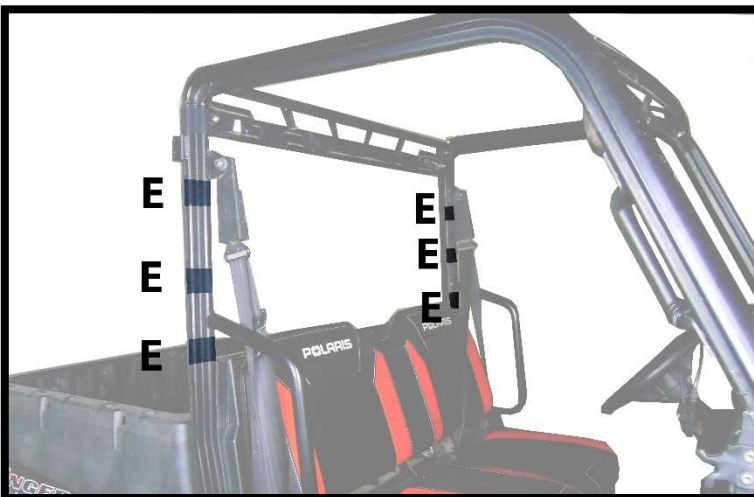
Figure 3: SHOWS PLACEMENT OF 6" VELCRO STRIPS (E)
