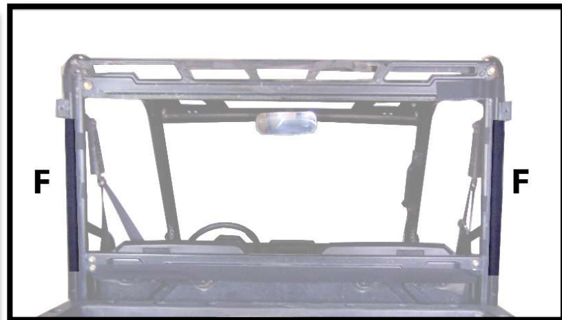
Figure 4: SHOWS PLACEMENT OF 18" VELCRO STRIPS (F).
