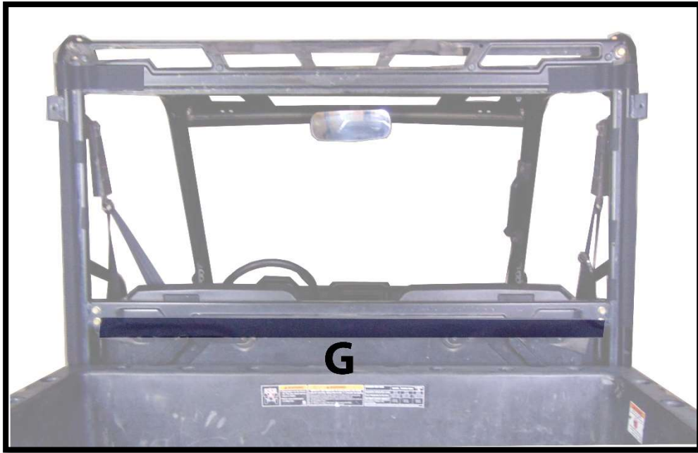
Figure 5: SHOWS PLACEMENT OF 54" VELCRO STRIP (G)
