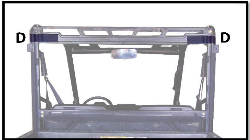
Figure 2: SHOWS PLACEMENT OF 12" VELCRO STRIPS (D).
