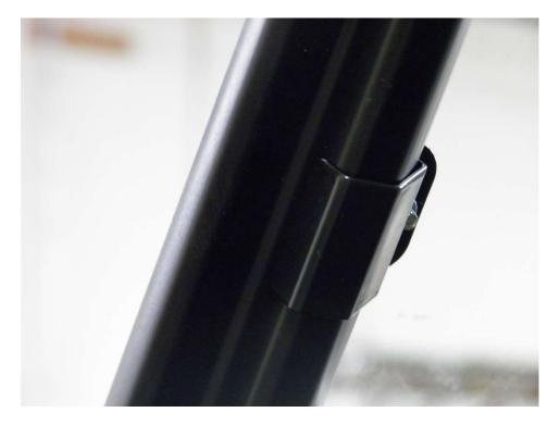
The threaded end of the clamp will sit under the windshield. The knob bolt with neoprene washer will go through the windshield and into the threads on the clamps. A nut will be inserted onto the knob bolt to hold in place.
