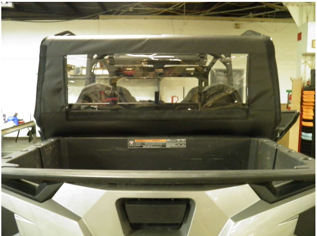
VELCRO IS SEWN DOWN THE SIDES OF THE BACK PANEL, THE DOOR KIT HAS TABS SEWN ON TO THE DOOR KIT THAT WILL STICK TO THIS VELCRO.
