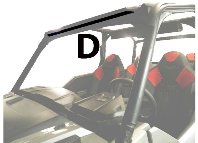
Figure 3: PLACE STRIP ALL THE WAY ACROSS THE VISOR. FOLD THE FRONT OF THE TOP CAP OVER THE FRONT OF THE VISOR AND ATTACH TO THE VELCRO.
