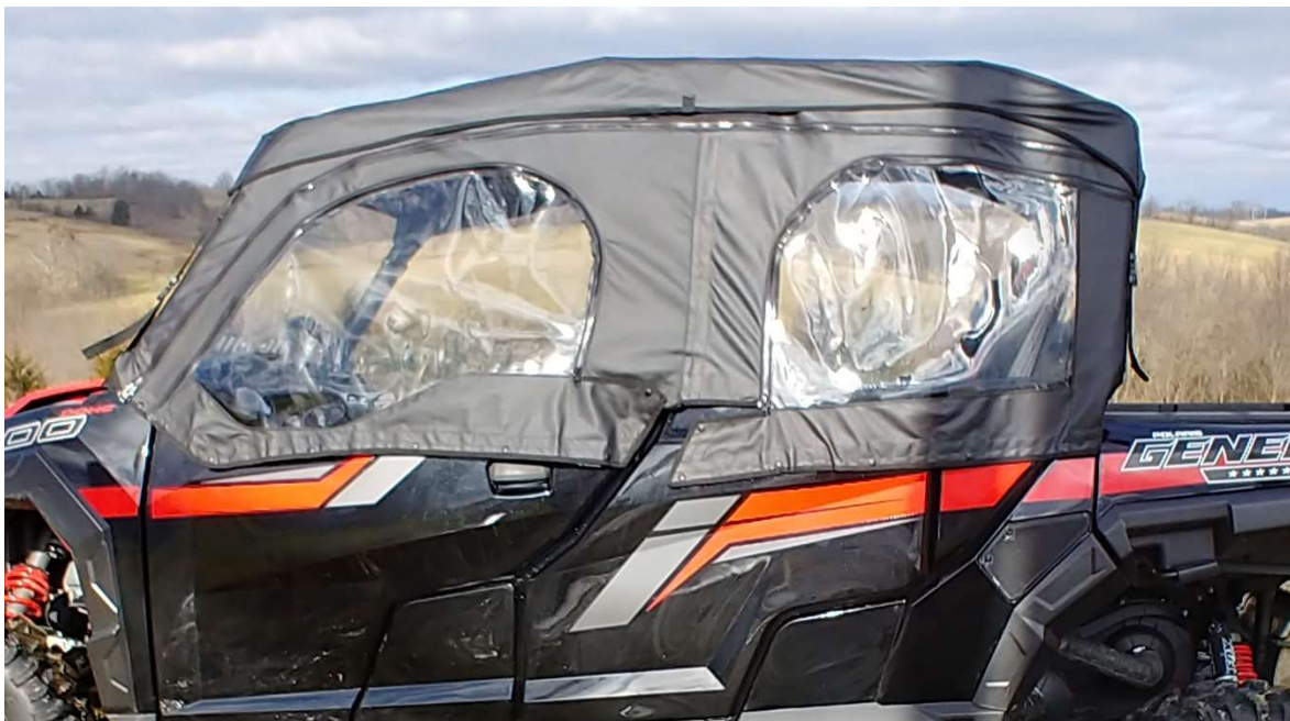
Figure 4: the strips placed along the outside of the door are optional. You may choose to install the snaps instead. Snaps will screw directly into the utv. Snaps should be installed after the doors are installed and are in the desired position. Snaps are permanent.
