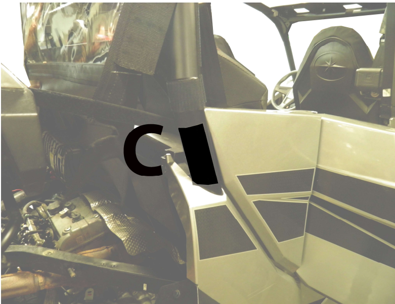
Figure 3: Shows placement of Velcro strip C, the drivers side will need a strip c as well.
