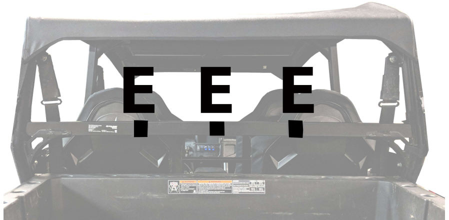
Figure 6: Shows placement of Velcro strips E.
