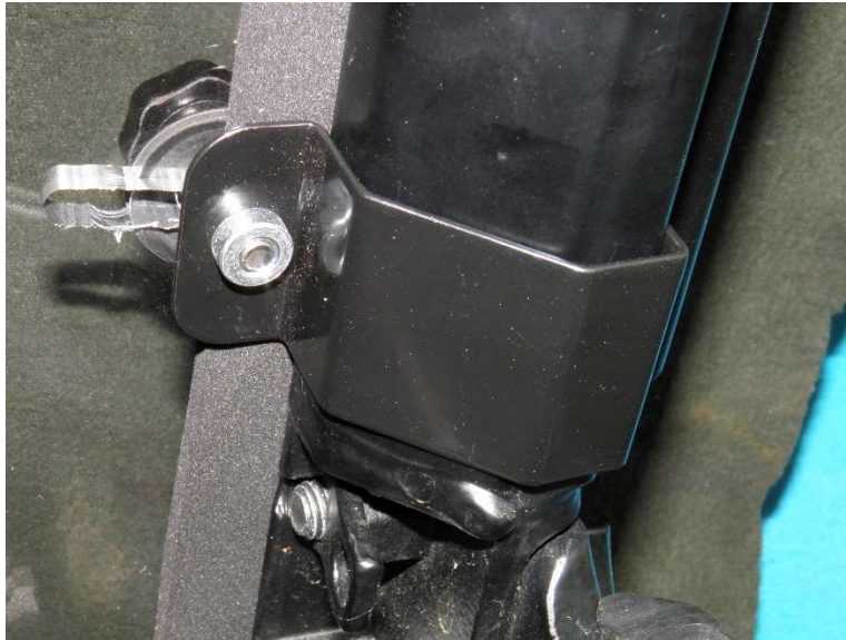
Interior view of angle clamp on roll bar
