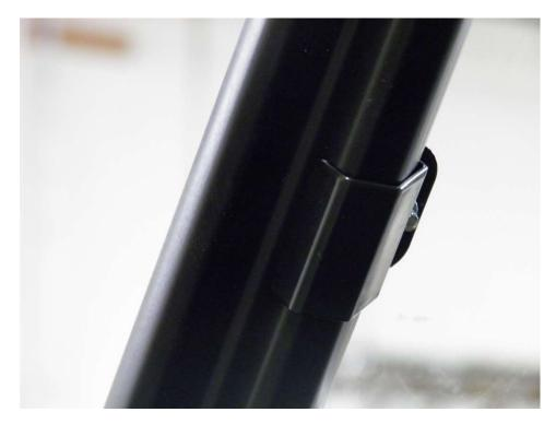
The threaded end of the clamp will sit under the windshield. The knob bolt with neoprene washer will go through the windshield and into the threads on the clamps. A nut will be inserted onto the knob bolt to hold in place.
