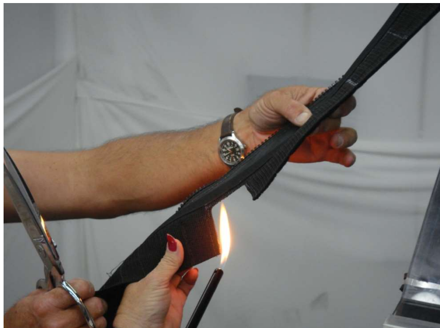
Seal Frayed Tab thread at the cut area using a lighter
