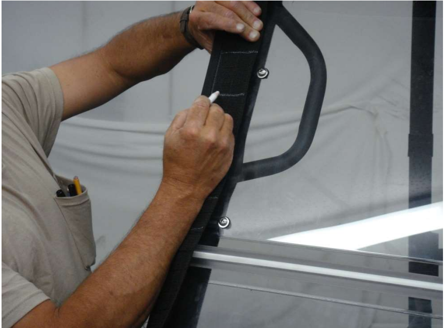
Mark windshield tabs where hard windshield clamps are located along the windshield Roll Bar
