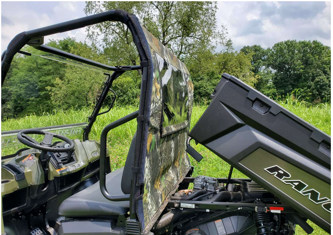
Figure 3: The double sided straps on either side of the back panel wrap around the roll bar and attach to themselves. You may choose to attach a little adhesive hook to help hold the back panel down but this is not necessary.
