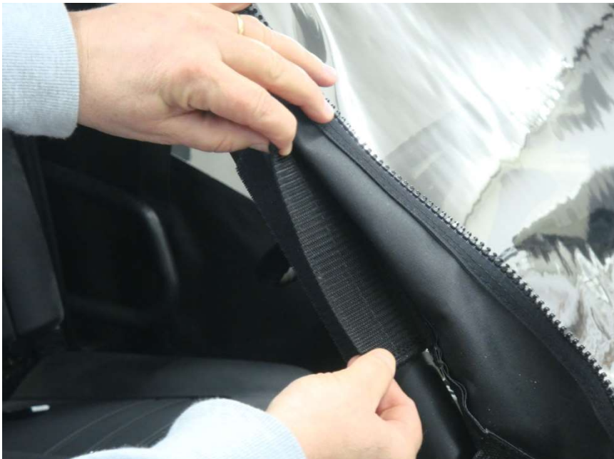
Figure 8.2 – attach Middle 10" Windshield Velcro Tabs
