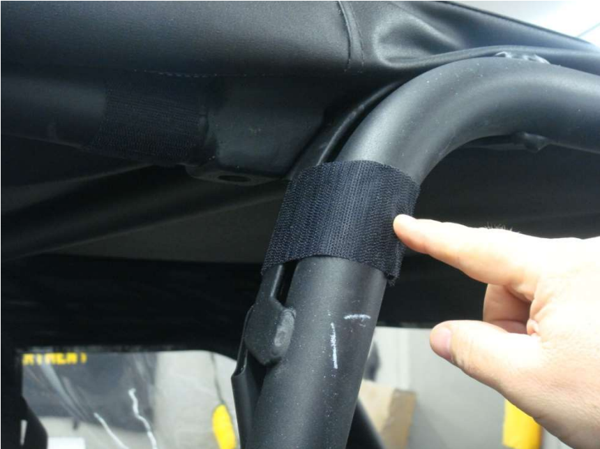
Figure 4.1 - install 11" Velcro Strips horizontally around Center Roll Bar uprights at the top
