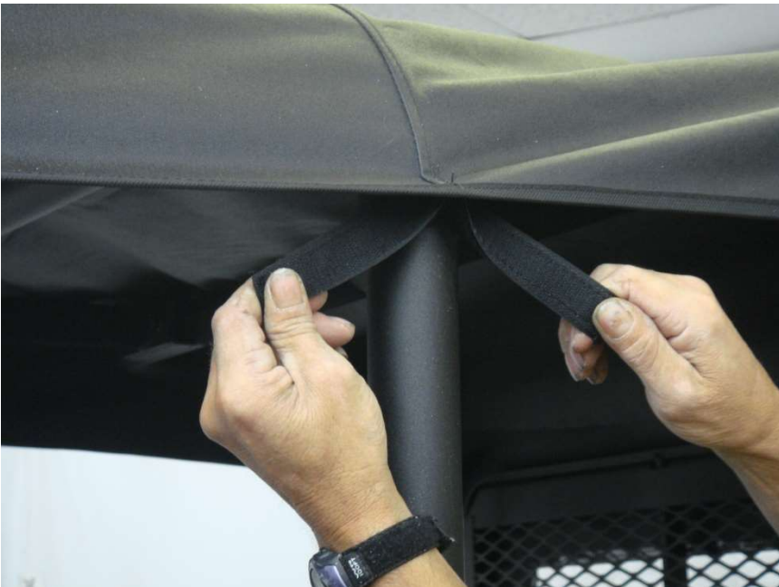
Figure 7.2 - attach Center Velcro tabs to installed 6" Velcro Strips
