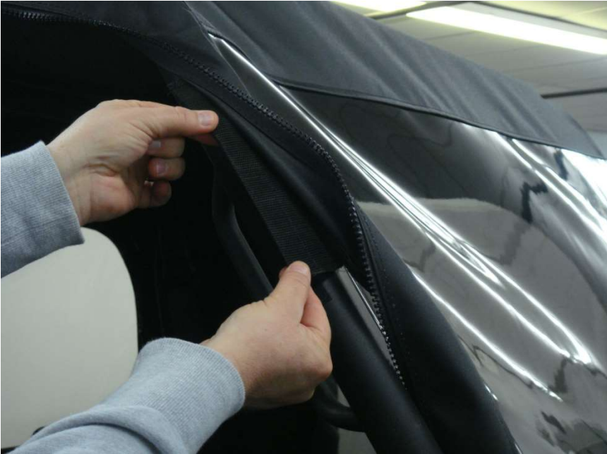
Figure 8.1 – attach Top 10" Windshield Velcro Tabs
