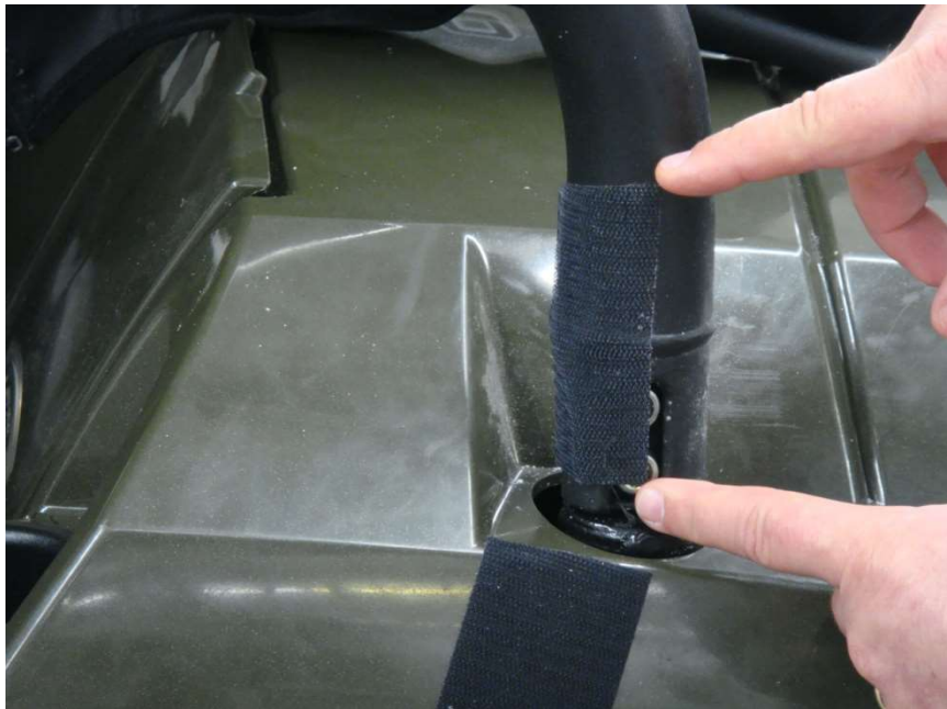
Figure 5.3 – install 5" Velcro Strips vertically along the bottom of the Front Windshield Roll Bar uprights
