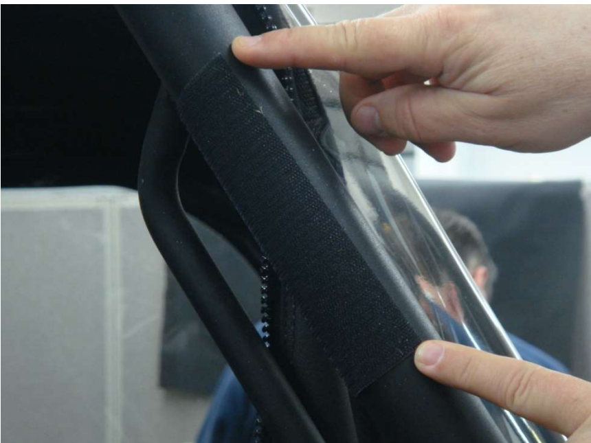
Figure 5.1 - install 10" Velcro strips vertically along the upper section of the front windshield Roll Bar upright
