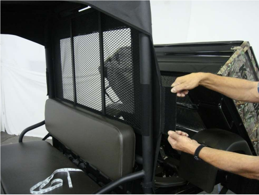
Figure 7.1 – attach rear Roll Bar Post upright 8" Velcro tabs
