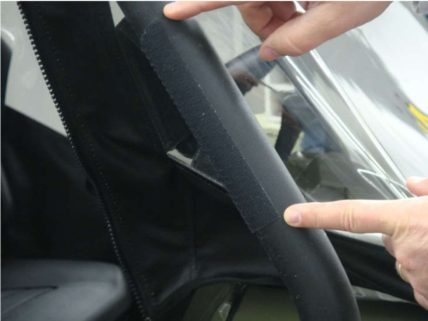
Figure 5.2 – install 10" Velcro strips vertically along the middle section of the Front Windshield Roll Bar uprights
