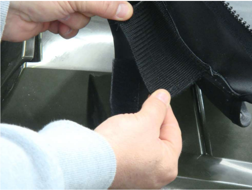
Figure 8.3 – attach bottom 5" Windshield Velcro tabs
