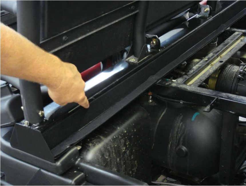
Figure 2.1 - attach 59" Velcro strips to Rear Cab Frame facing toward the rear of the vehicle
