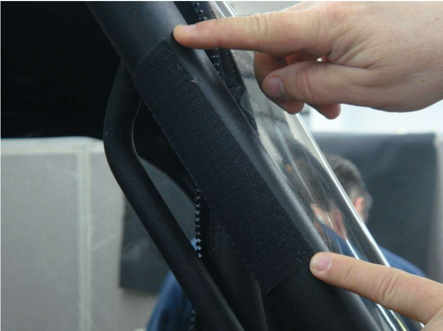
Install 10" Velcro strips vertically along the upper section of the front windshield Roll Bar upright
