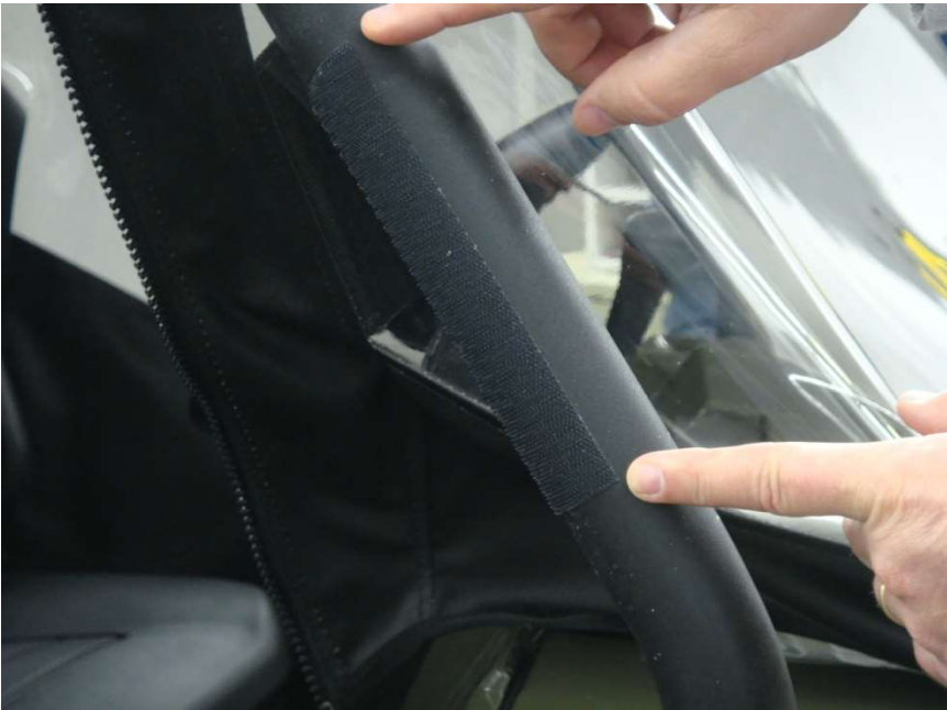
Install 10" Velcro strips vertically along the middle section of the Front Windshield Roll Bar uprights
