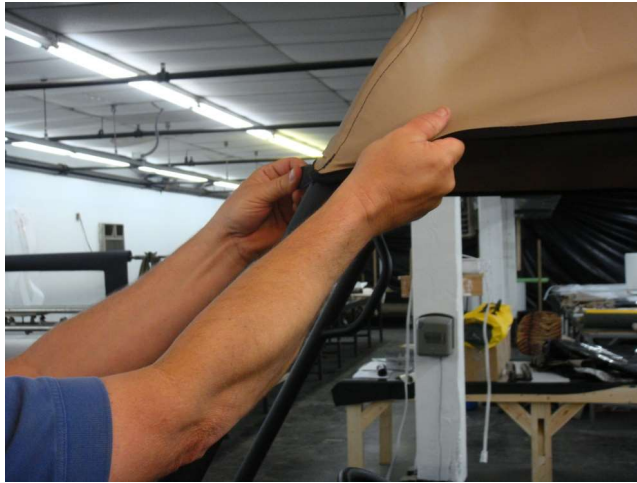
Figure 4.1 - Attach front, center and rear Enclosure Velcro tabs to installed Velcro strips
