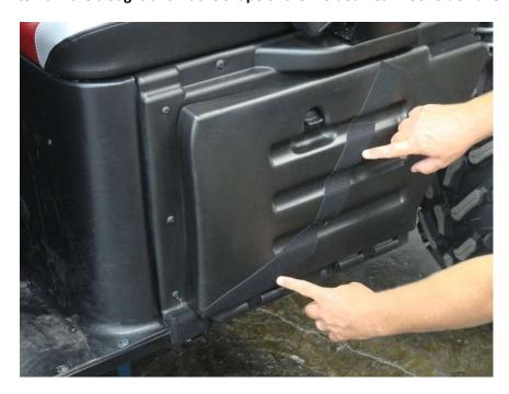
Figure 8.1 - Install 19.5" and 10" Velcro Strips on the Rear Door Side Panel
