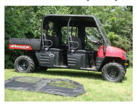
Figure 18.1 - Top Cap should fit snuggly along the vehicle Top Roll Bar Structure
