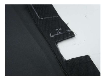
Figure 14.2 - DO NOT CUT VELCRO TAB BINDING STITCHES ATTACHING BINDING TO THE ENCLOSURE – stay back at least ½" from Stitching while Cutting
