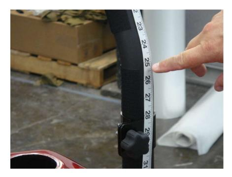
Figure 6.2 - install 12" Velcro strips along the inside edge of the front windshield Roll Bar upright lower section
