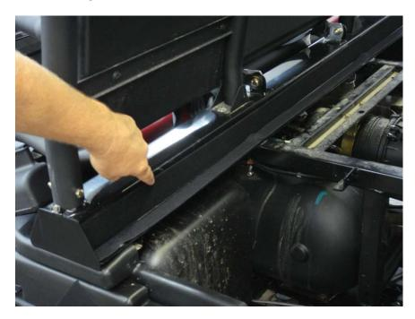
Figure 2.1 - attach 59" Velcro strip to Rear Cab Frame facing toward the rear of the vehicle
