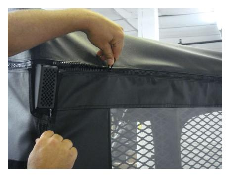
Figure 11.1 - attach Rear Panel onto Top Cap panel by Zipping the panels together
