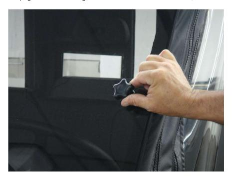
Figure 17.1 - Tighten Windshield Quick Connect Knobs
