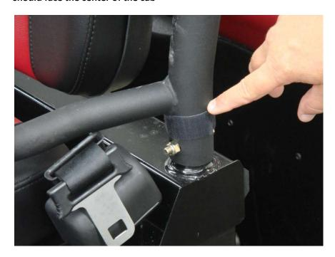
Figure 5.1 - install 6" (1" wide) Velcro strips horizontally around the bottom of the Center Roll Bar Uprights
