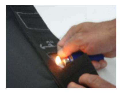
Figure 14.3 - With a lighter briefly melt the frayed ends of the fabric to prevent future fraying of the material
