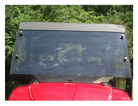
Figure 16.2 - Leading Windshield edge of enclosure should extend ¼" over the installed Windshield Velcro Strip so it is completely hidden.
