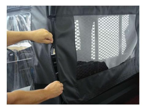
Figure 19.2 - attach Side Door Panels by Zipping them to the Rear Panel
