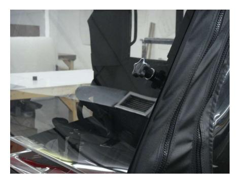
Figure 15.1 - Attach front Windshield Velcro Tabs to installed Velcro strips – Enclosure binding should fit tight against the windshield edge
