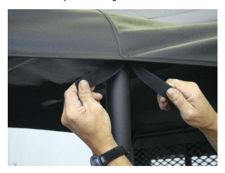
Figure 10.1 - attach Top Cap Center and Rear upper Velcro tabs to installed 6" Velcro Strips
