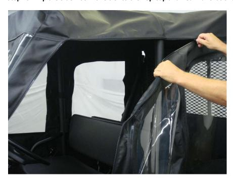
Figure 19.1 - Attach Side Door Panels by zipping them to the Top Cap
