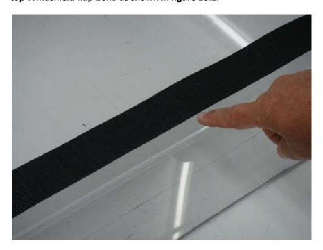
Figure 16.1 - Install the 60" Polycarbonate Windshield Velcro Strip below the Top Windshield Flap Bend
