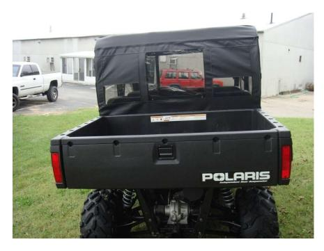
Figure 18.2 – Rear Panel should fit tightly across the back of the vehicle
