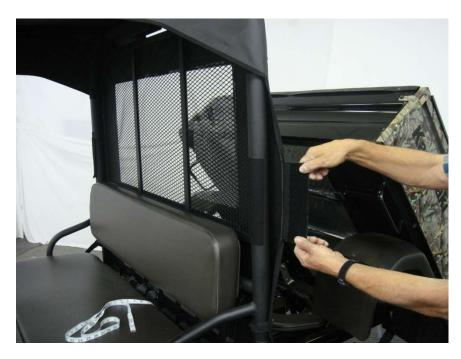
Figure 11.3 – attach 8" Rear Panel Roll Bar upright tabs to installed Velcro Strips
