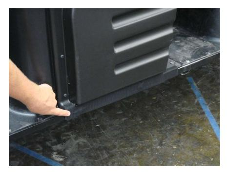
Figure 9.1 - attach 15" Velcro Strips to side Rocker Panels between the Front and Rear Doors
