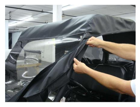
Figure 13.1 – attach Top and Middle 10" and Bottom 5" Windshield Velcro Tabs
