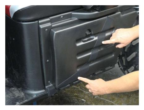
Figure 8.1 - Install 19.5" Velcro Strips on the Rear Door Side Panel
