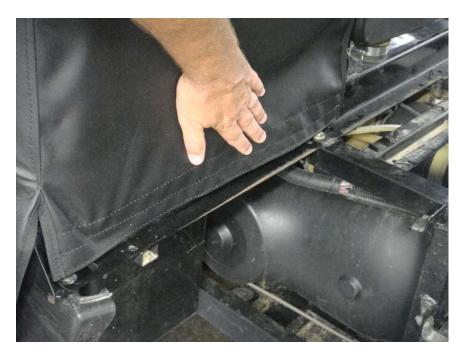
Figure 12.2 – Square Enclosure to Rear of Cab Frame and press Enclosure Velcro Tab onto 59" installed Velcro Strip
