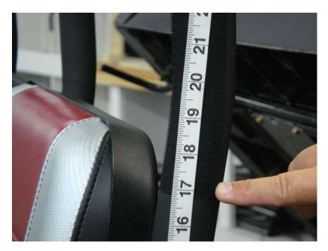
Figure 3.1 attach 8" Velcro strips vertically on the Rear Roll Bar uprights
