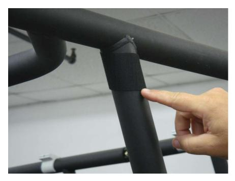
Figure 4.1 - install 6" Velcro Strips horizontally around Center Roll Bar uprights
