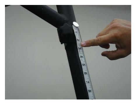
Figure 6.1 - install 10 " Velcro strips vertically along the Top of the front windshield Roll Bar upright
