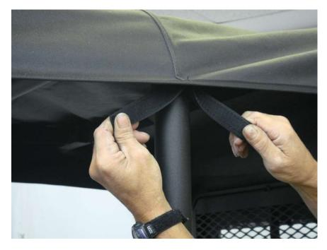
Figure 11.1 - attach Top Cap Center and Rear upper Velcro tabs to installed 6" Velcro Strips
