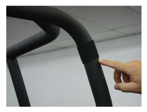
Figure 4.2 – install 6" Velcro strips horizontally around Rear Roll Bar Uprights
