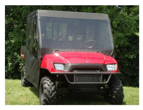
Figure 17.1 - Enclosure and Polycarbonate should fit as shown
