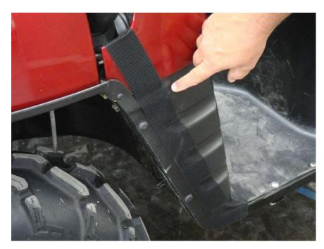
Figure 7.1 – attach 19" Velcro strips Vertically to the lower section of the Dash Cowl side panel and 4" strips horizontally at the bottom
