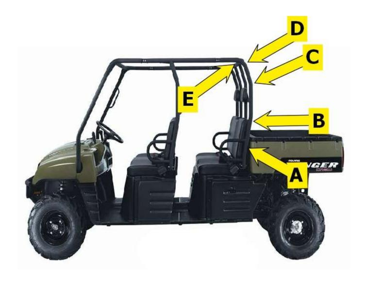
**Step 5:** Begin attaching the rear panel to the cab frame by attaching the sewn-in Velcro loop at the bottom of the rear panel.
