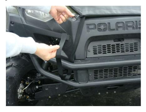
Figure 5.1 – guide front Hood straps around bumper
