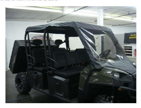
**Step 4:** Pull the enclosure (each side of the front windshield) downward toward the front of the vehicle and attach the 8" and 6" webbing/loop tabs to the corresponding adhesive hook strips on the front roll bar uprights. Reposition the webbing/loop tabs to square the windshield to the cab frame.
