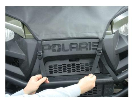
Figure 5.3 – Tighten Hood Straps by pulling down on the strap below the buckle
