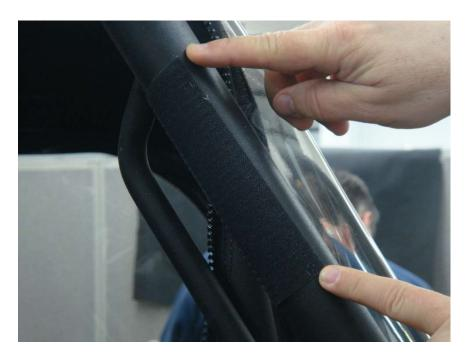
Reference D & E-Install adhesive hook strips vertically along the outside edge of the front roll bar uprights.
