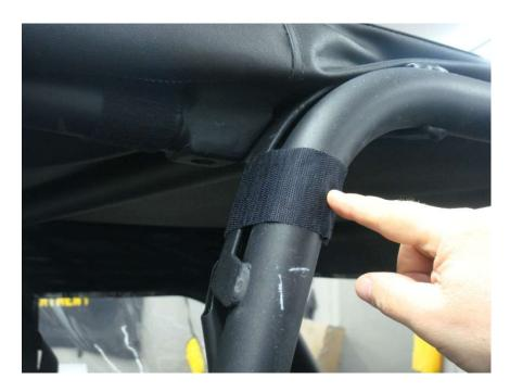
Reference A, B, and C-wrap adhesive hook strips horizontally around roll bars.
