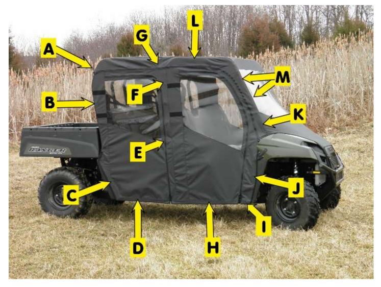
**Step 4:** After all adhesive Velcro strips are attached, begin attaching enclosure by first squaring the back of the enclosure to the rear of the cab frame and attaching the sewn-in Velcro loop to the 54" adhesive strip at the base of the back panel.
