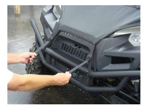
**Step 8:** Cut the webbing strip with household scissors. **AGAIN, DO NOT CUT INTO THE BINDING.** Seal the frayed edges with a lighter. Have a wet cloth handy to dab the edges.
