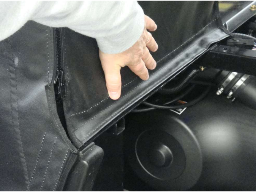
Figure 7.2 – Square back of enclosure to vehicle rear cab frame and attach 21” Velcro Tabs
