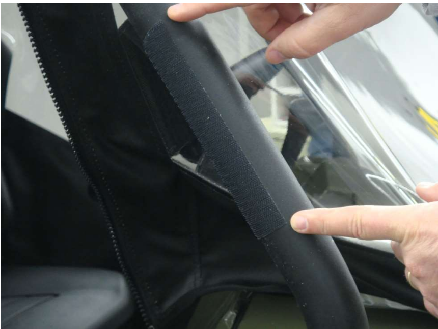
Figure 6.2 – install 6" Velcro strips vertically along the middle section of the Front Windshield Roll Bar uprights
