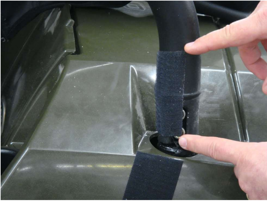
Figure 6.3 – install 4” Velcro Strips vertically along the bottom of the Front Windshield Roll Bar uprights
