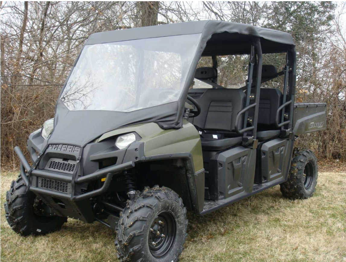
Figure 10.1 - Enclosure should fit snug along the vehicle Top Roll Bar Structure and Windows should not have major wrinkles.
