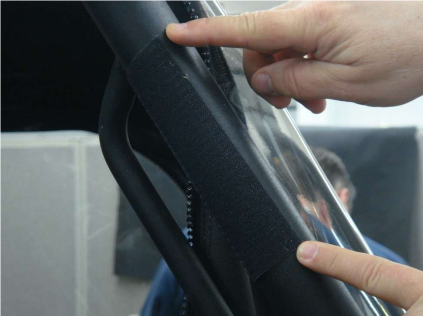
Figure 6.1 - install 8" Velcro strips vertically along the upper section of the front windshield Roll Bar upright
