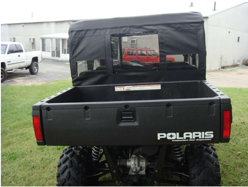
Figure 10.2 – Rear Panel should fit tightly across the back of the vehicle
