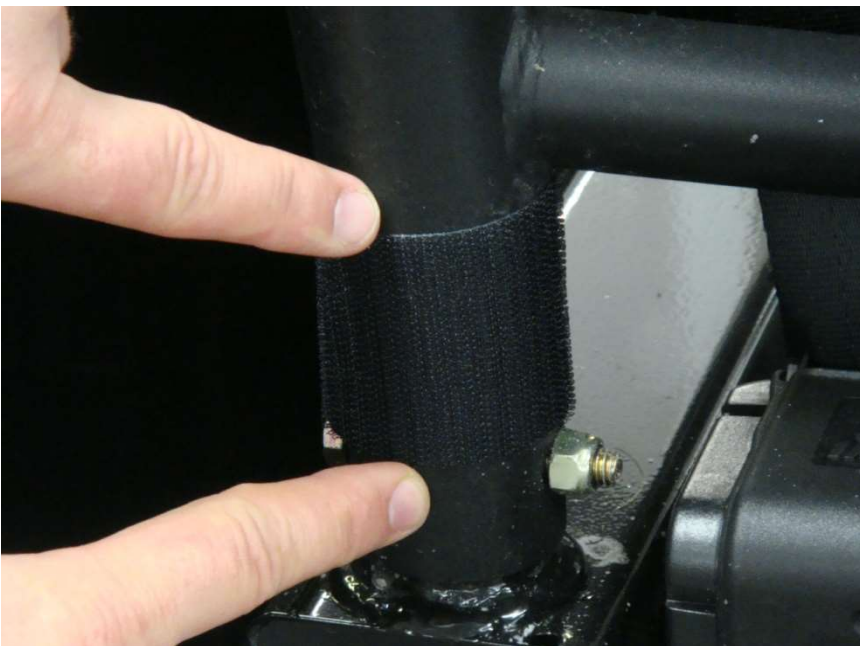
Figure 5.1 - install 6" Velcro strips horizontally around the bottom of the Rear Roll Bar Uprights
