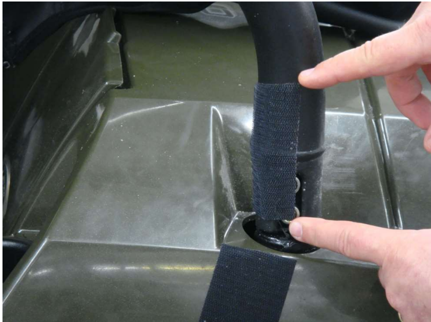
Figure 3.3 – install 4" Velcro Strips vertically along the bottom of the Front Windshield Roll Bar uprights
