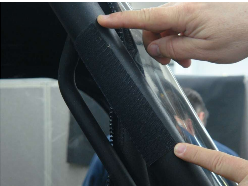
Figure 3.1 - install 8" Velcro strips vertically along the upper section of the front windshield Roll Bar upright
