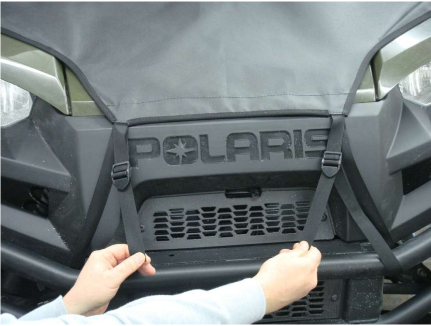
Figure 6.3 – Tighten Hood Straps by pulling down on the strap below the buckle
