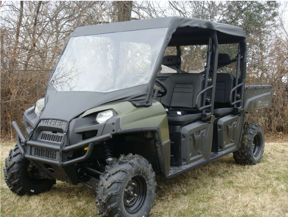
Figure 7.1 - Enclosure should fit snugly along the vehicle Top Roll Bar Structure and should not have major wrinkles.
