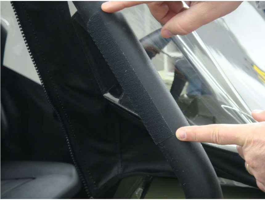
Figure 3.2 – install 6" Velcro strips vertically along the middle section of the Front Windshield Roll Bar uprights
