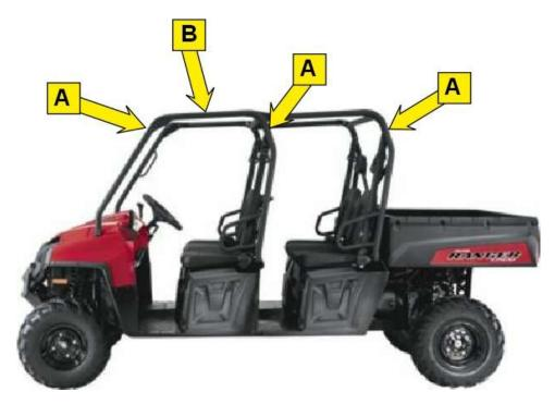
**Step 4:** Pull the top down tightly on the two front roll bars and two middle roll bars keeping the side seams aligned with the outside edge of the side roll bars. Wrap the double-sided straps around the attached Velcro strips.
