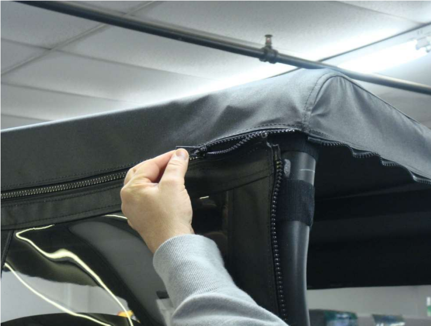
Figure 11.1 - attach Rear Panel onto Top Cap panel by zipping the panels together
