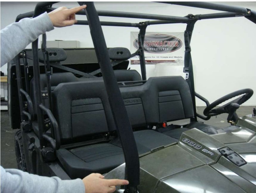
Figure 6.1 - install 23" Velcro strips along the inside edge of the front windshield Roll Bar upright upper section and 5" Velcro strips along the front windshield lower section just below the roll bar bend.
