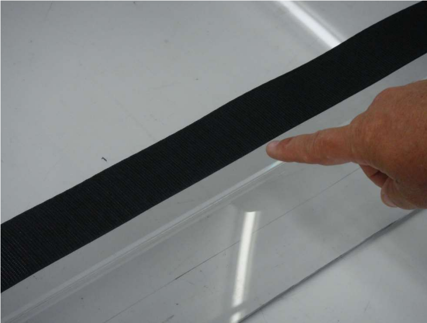
Figure 16.1 - Install the 53" Polycarbonate Windshield Velcro Strip below the Top Windshield Flap Bend
