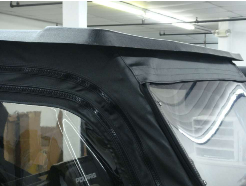
Figure 16.2 - Leading Windshield flap edge of enclosure should extend \frac{1}{4} " over the installed Windshield Velcro Strip so it is completely hidden.
