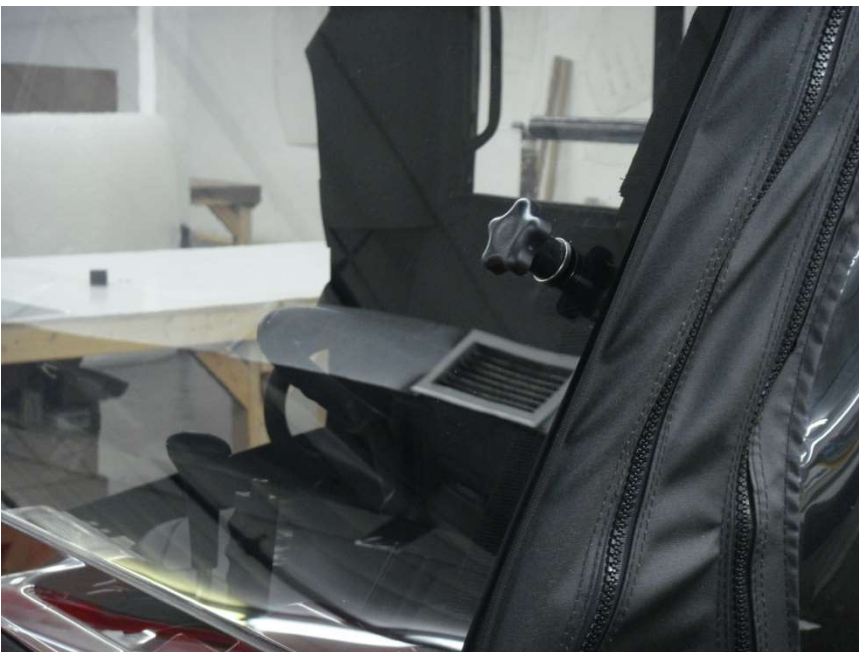
Figure 15.1 - Attach front Windshield Velcro Tabs to installed Velcro strips – Enclosure binding should fit tight against the windshield edge
