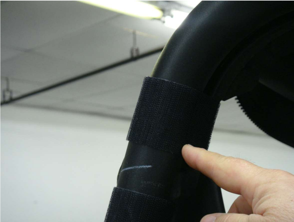
Figure 5.2 - install 10" Velcro strips horizontally around the top of the Rear Roll Bar Uprights
