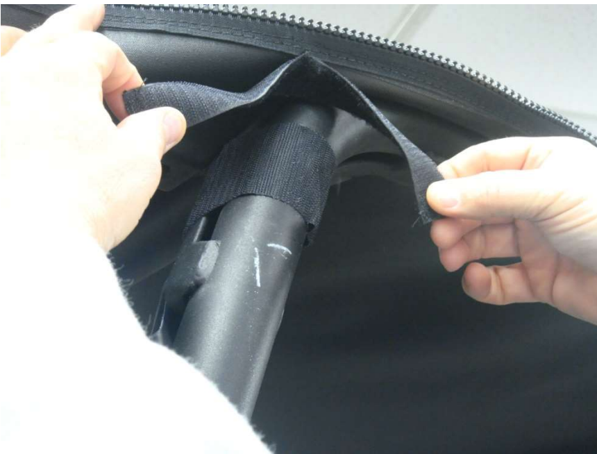
Figure 10.2 - attach Top Cap Center Roll Bar upright and Rear Top Velcro upright tabs to installed 10" Velcro Strips
