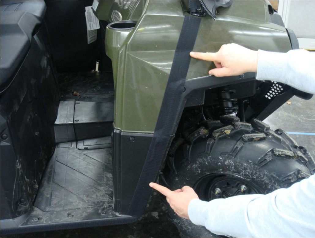
Figure 7.1 – attach 28 1/2" Velcro strips vertically to the lower section of the Dash Cowl side panel and 3 1/2" strips horizontally at the bottom
