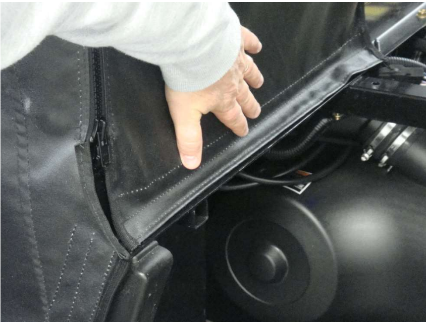
Figure 11.2 – Square Enclosure to Rear of Cab Frame and press Enclosure Velcro Tab onto 21" installed Drivers side and Passenger's side Velcro Strips
