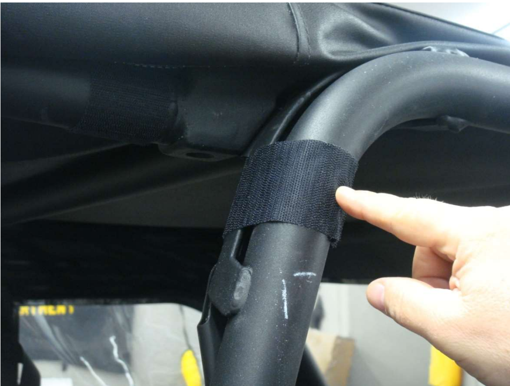
Figure 5.1 - install 10" Velcro strips horizontally around the top of the Center Roll Bar Uprights
