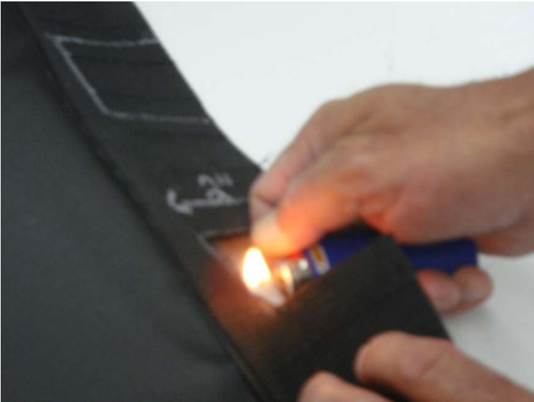
Figure 14.3 - With a lighter briefly melt the frayed ends of the fabric to prevent future fraying of the material
