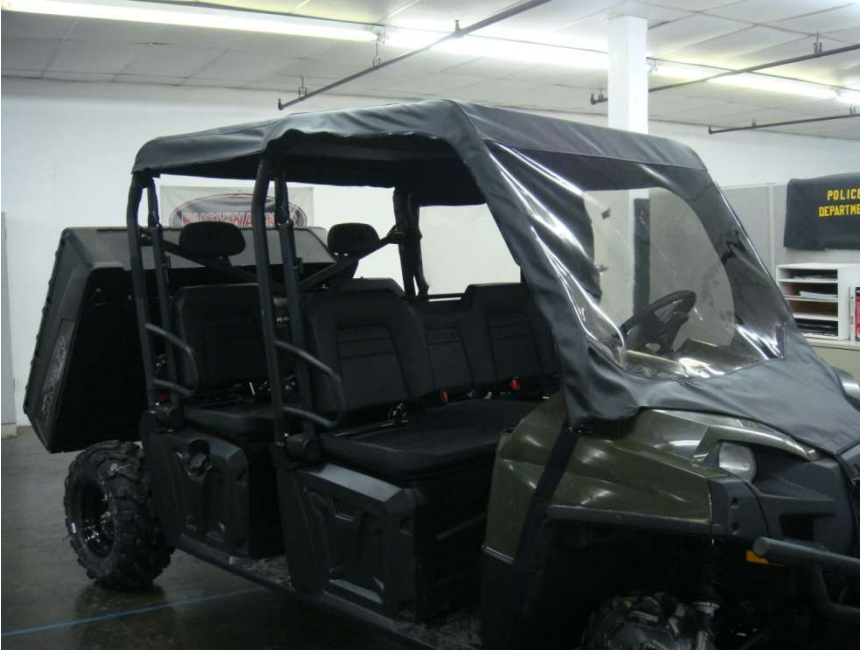
Figure 10.1 – lay top cap on vehicle and align seams with center top roll bar cross-members.
