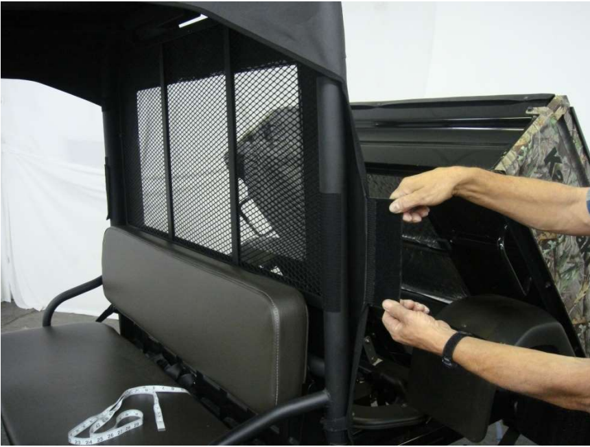
Figure 10.3 – attach 8" Rear Panel Roll Bar upright tabs to installed Velcro Strips
