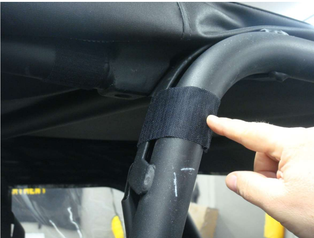
Figure 3.1 - install 9" Velcro strips horizontally around the top of the Center Roll Bar Uprights
