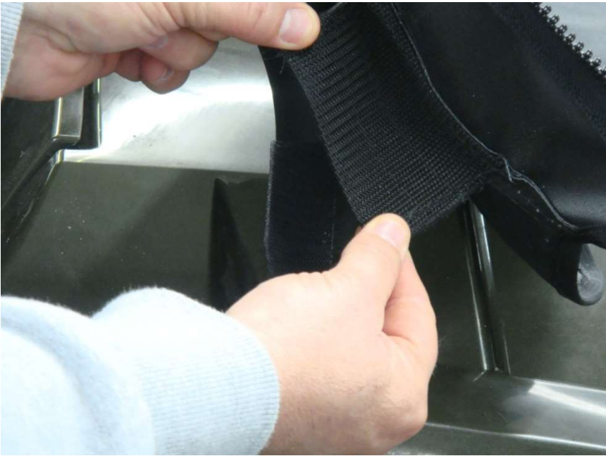
Figure 11.3 – attach bottom 4” Windshield Velcro tabs
