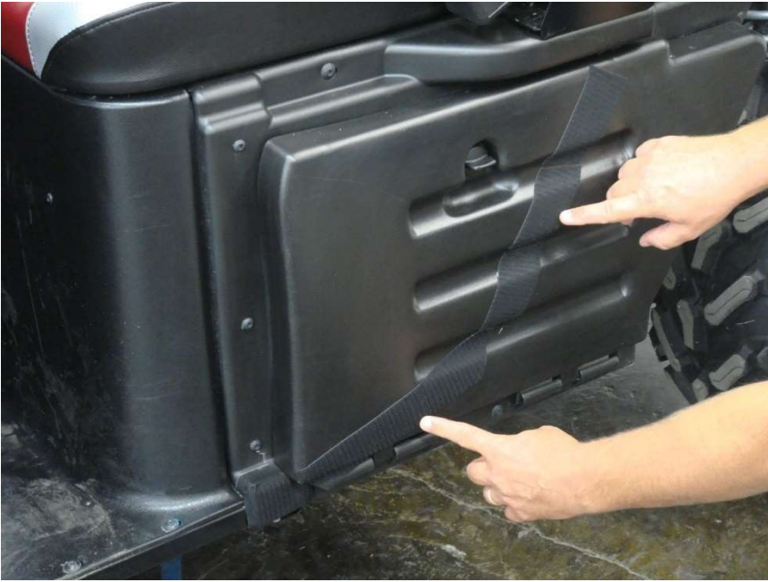
Figure 8.1 - Install 18.5" Velcro Strips on the Rear Door Side Panel
