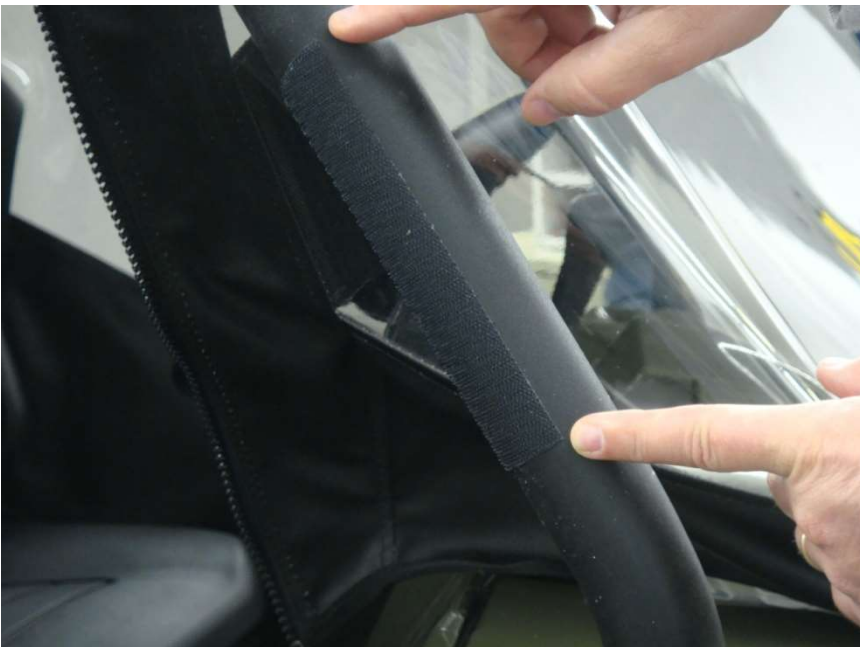
Figure 6.2 - install 6" Velcro strips vertically along the middle of the front windshield Roll Bar upright
