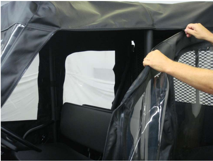
Figure 13.1 - Attach Side Door Panels by zipping them to the Top Cap and Rear Panel
