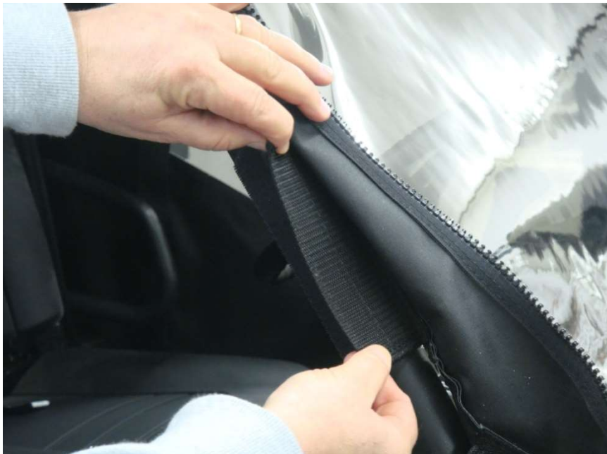
Figure 11.2 – attach Middle 6" Windshield Velcro Tabs
