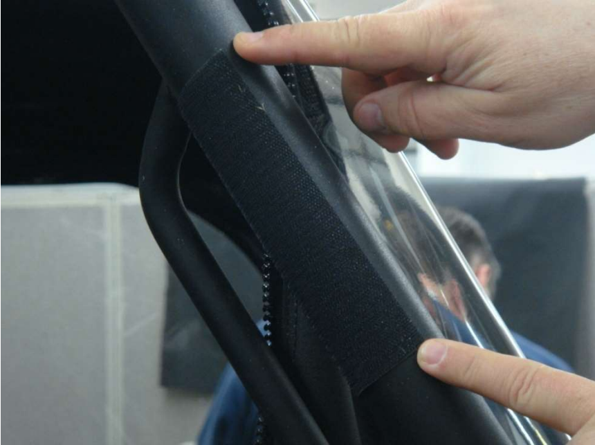
Figure 6.1 - install 8" Velcro strips vertically along the Top of the front windshield Roll Bar upright
