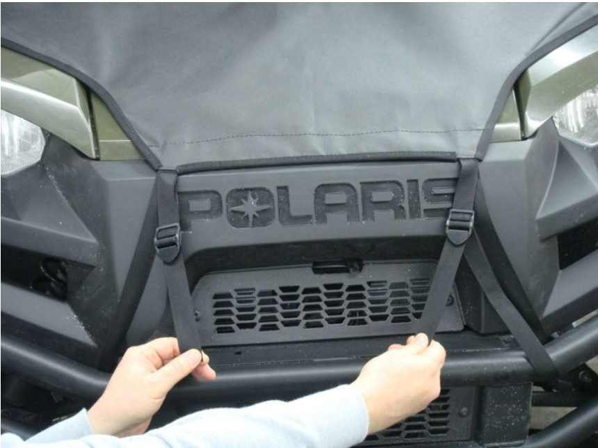
Figure 12.3 – Tighten Hood Straps by pulling down on the strap below the buckle
