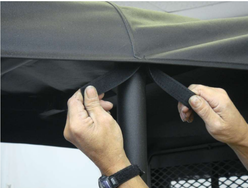
Figure 10.4 - attach Top Cap Center and Rear upper Velcro tabs to installed 6" Velcro Strips
