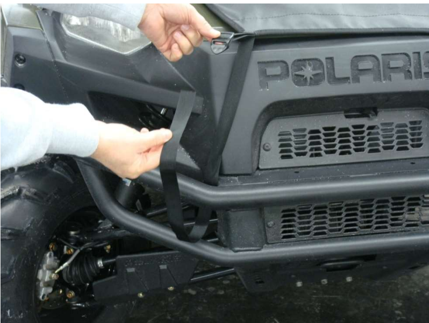
Figure 12.1 – guide front Hood straps around bumper
