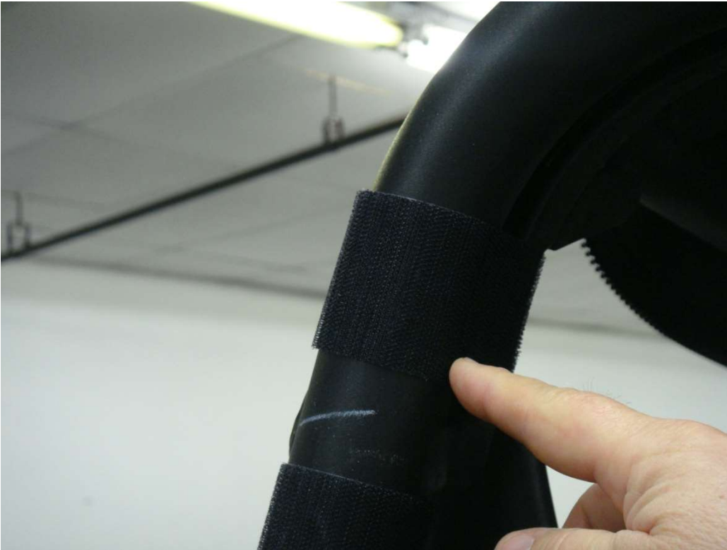
Figure 3.2 - install 9" Velcro strips horizontally around the top of the Rear Roll Bar Uprights
