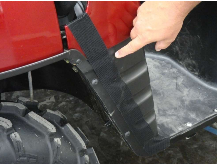
Figure 7.1 – attach 19” Velcro strips Vertically to the lower section of the Dash Cowl side panel and 4” strips horizontally at the bottom
