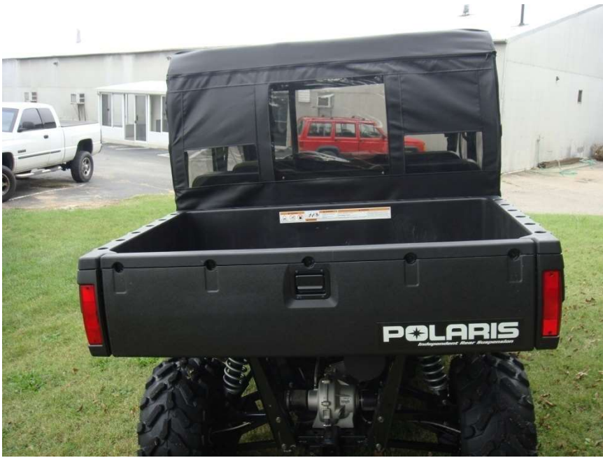
Figure 15.2 – Rear Panel should fit tightly across the back of the vehicle
