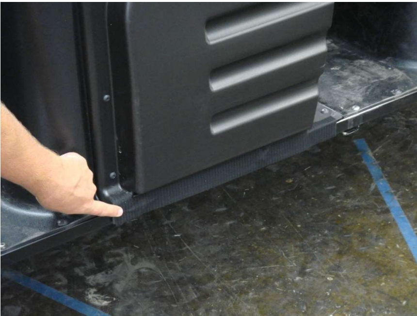
Figure 9.1 - attach 15" Velcro Strips to side Rocker Panels between the Front and Rear Doors
