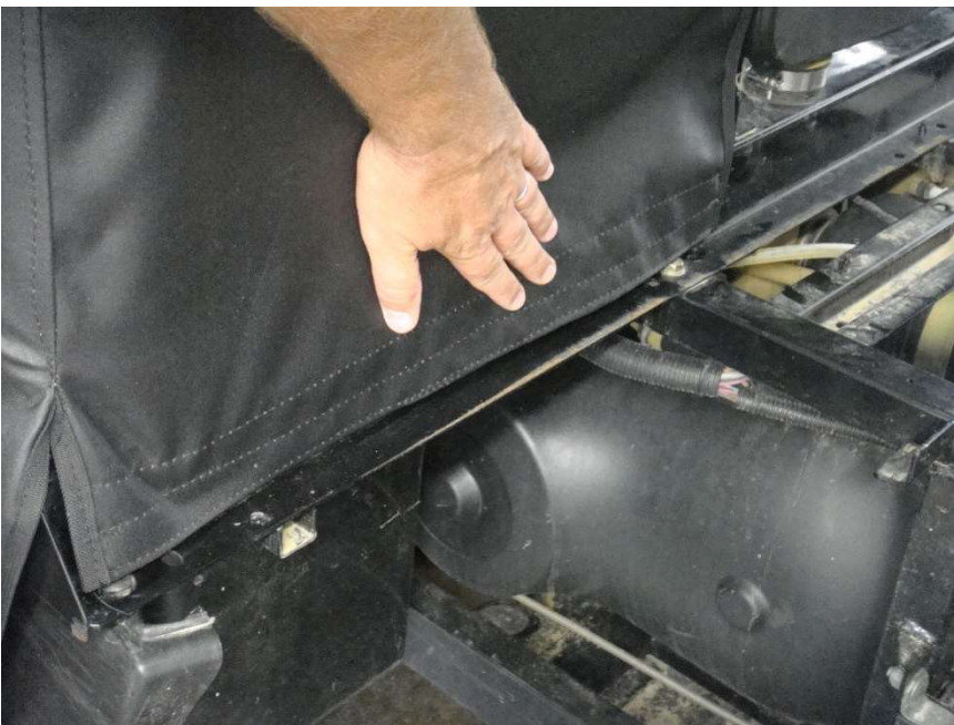
Figure 10.2 – Square Enclosure to Rear of Cab Frame and press Enclosure Velcro Tab onto the 2-21" installed Velcro Strips
