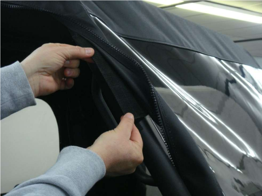
Figure 11.1 – attach Top 8" Windshield Velcro Tabs
