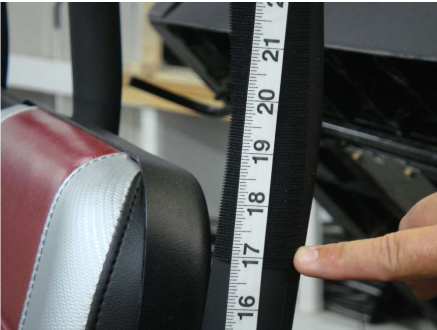
Figure 4.1 attach 8" Velcro strips vertically on the Rear Roll Bar uprights
