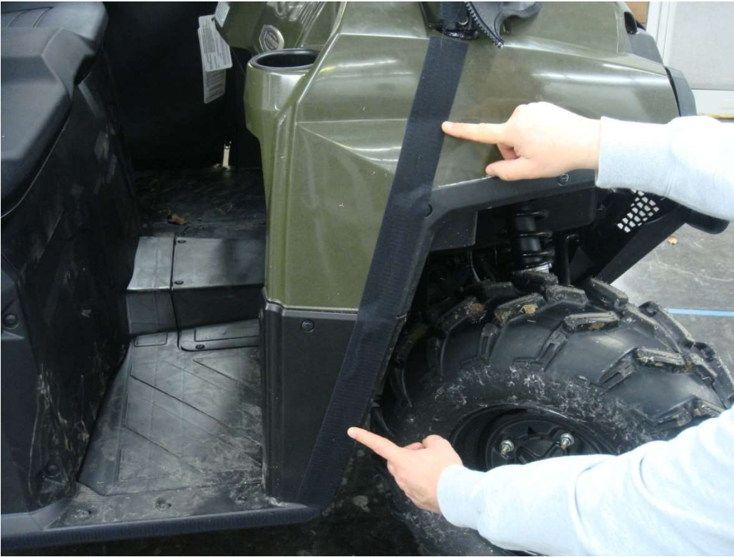
Attach 28 1/2" Velcro strips vertically to the lower section of the Dash Cowl side panel
