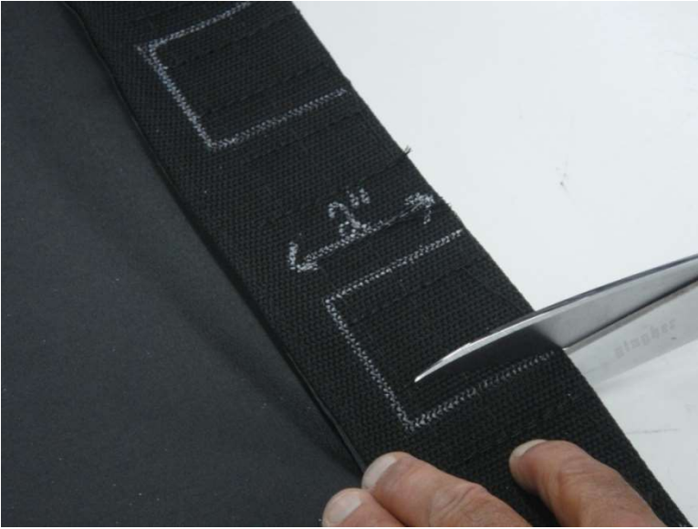
Figure 7.1 Cut out Velcro Tab Binding at each Clamp Location
