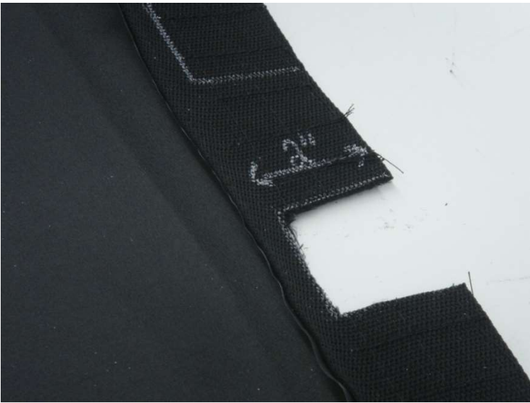
Figure 7.2-DO NOT CUT VELCRO TAB BINDING STITCHES ATTACHING BINDING TO THE ENCLOSURE – stay back at least ½” from Stitching while Cutting
