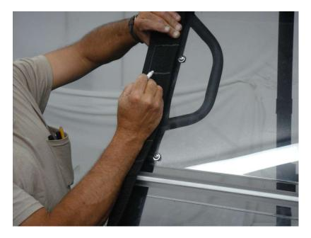
**Step 8:** Cut the webbing strip with household scissors. **AGAIN, DO NOT CUT INTO THE BINDING.** Seal the frayed edges with a lighter. Have a wet cloth handy to dab the edges if needed.
