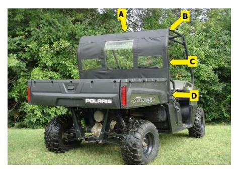
**Step 2:** With the help of an assistant, hold the back panel squarely to the cab frame. Not the location of the sewn-in Velcro loop strips. The adhesive Velcro hook strips will be placed on the cab frame to correspond to the sewn-in strips. Take a moment to note the location of the sewn-in Velcro loop.
