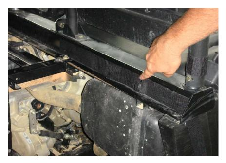
**Step 5:** After all adhesive Velcro hook strips are attached to the cab frame, place the back panel on the cab frame and attach the sewn-in Velcro loop strips to the adhesive strips.
