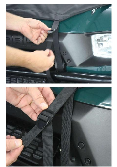
Repeat all steps necessary to align and tighten the enclosure to the cab frame.
