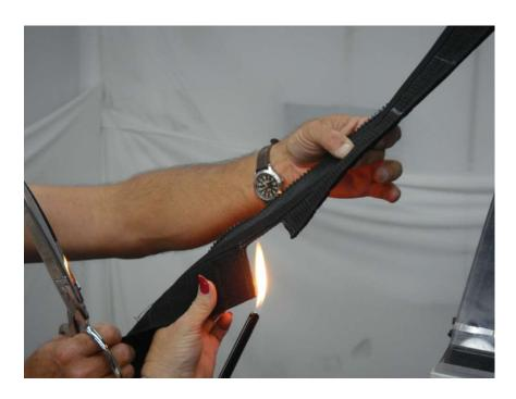
Seal Frayed Tab thread at the cut area using a lighter
