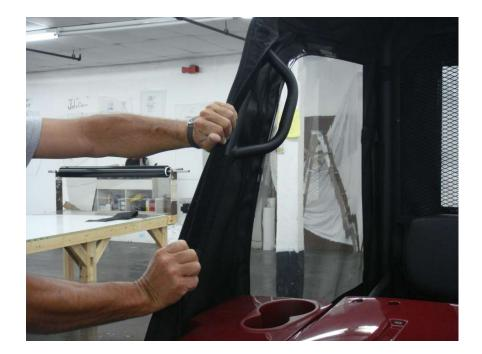
**Step 7:** The webbing/Velcro strip that runs the length of the front roll bars will need to be cut to accommodate the windshield clamps and the grab handle. With chalk, mark the webbing strip where cuts will be made. **DO NOT CUT INTO THE BINDING.**
